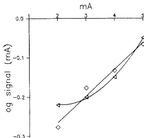
Figure 6. OG signal for  $1s_5 \rightarrow 2p_2$  (□) and  $1s_5 \rightarrow 2p_4$  (Δ) transition.
