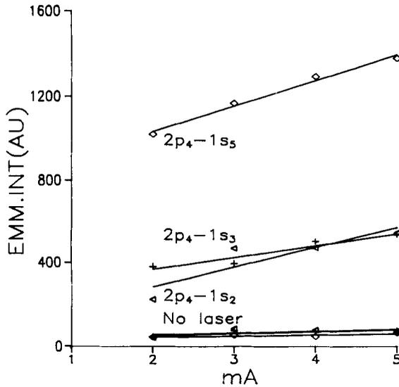
Figure 5. Dependence of the emission intensity for  $2p_4 \rightarrow 1s_i$  ( $i = 2, 4, 5$ ) transitions on discharge current.
