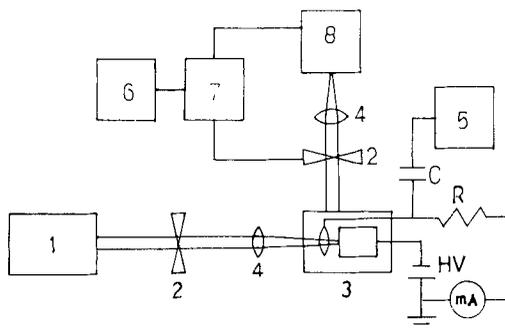
**Figure 1.** Experimental set-up (1. single mode ring dye laser, 2. chopper, 3. Ne-Mo hollow cathode, 4. lens, 5. CRO, 6. computer, 7. lock-in amplifier, 8. monochromator,  $R = 45 \text{ K}\Omega$ ,  $C = 0.1 \mu\text{F}$ ).
