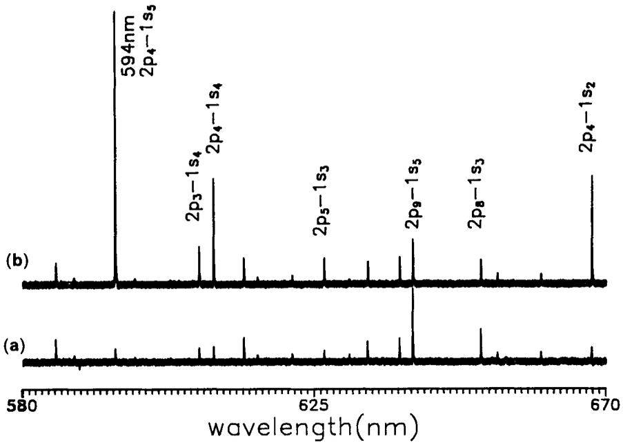
Figure 4. a) Emission spectrum of neon discharge at 5 mA and b) the same under laser irradiation at 594.5 nm.
