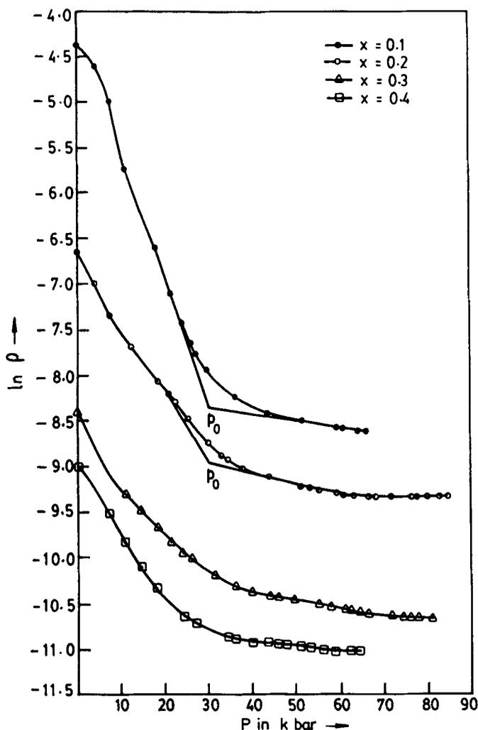
Figure 1. The behaviour of electrical resistivity of  $\text{SmSe}_{1-x}\text{As}_x$  as a function of pressure.
