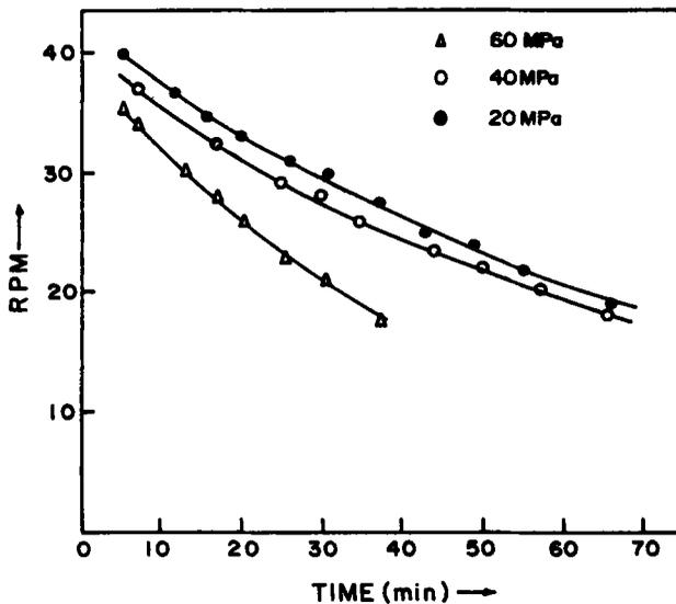
**Figure 3.** Deceleration rate of the piston with time operating at different applied pressures.
