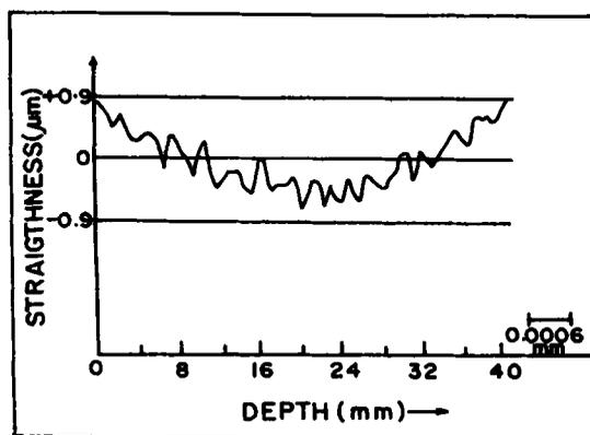
**Figure 4.** Dimensional measurement of straightness of the piston along its length of  $40 \text{ mm}$ . (Magnification 16300).
