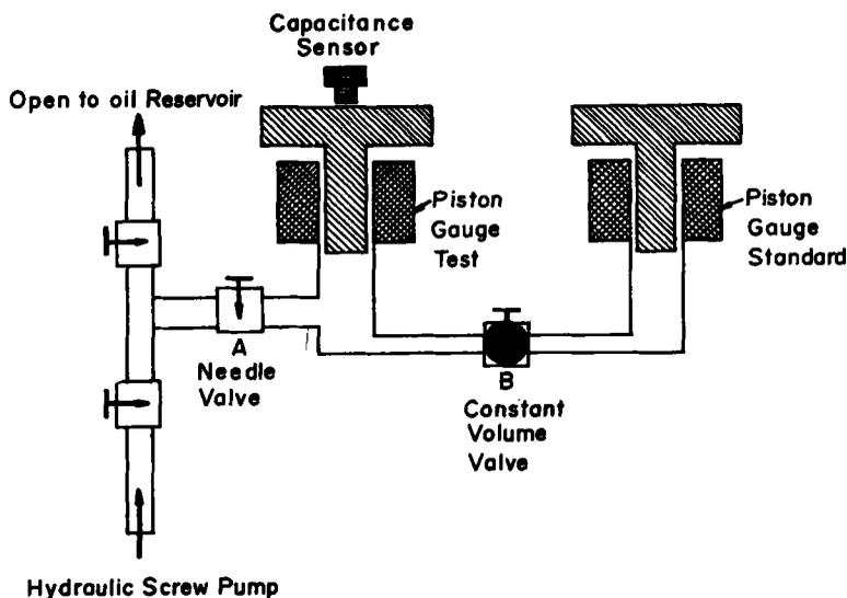
Figure 2. Experimental crossfloat arrangement between the test gauge and the standard piston gauge.
