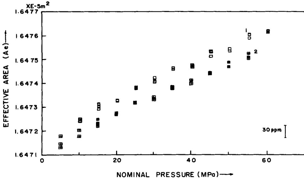
Figure 7. Effective area  $A_e$  of NPL-60 obtained by direct crossfloating against NPL-140 (1) and by crossfloating against NPL-100(2).
