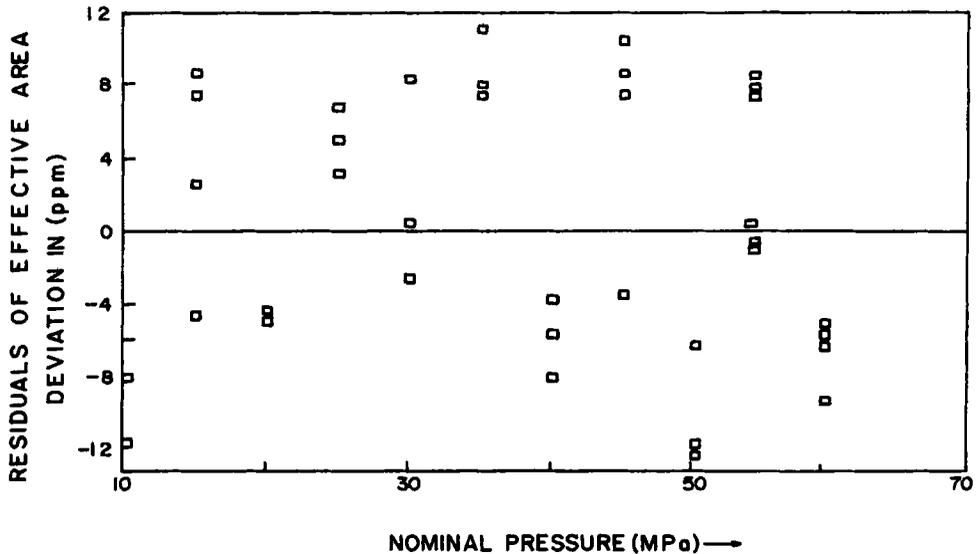
Figure 6. Deviation of measured values of the effective area of NPL-60 from the best linear fit  $A_e = 1.647188 \text{ E-5} (1 + 4.4 \text{ E-12} P)$  when calibrated by NPL-140.
