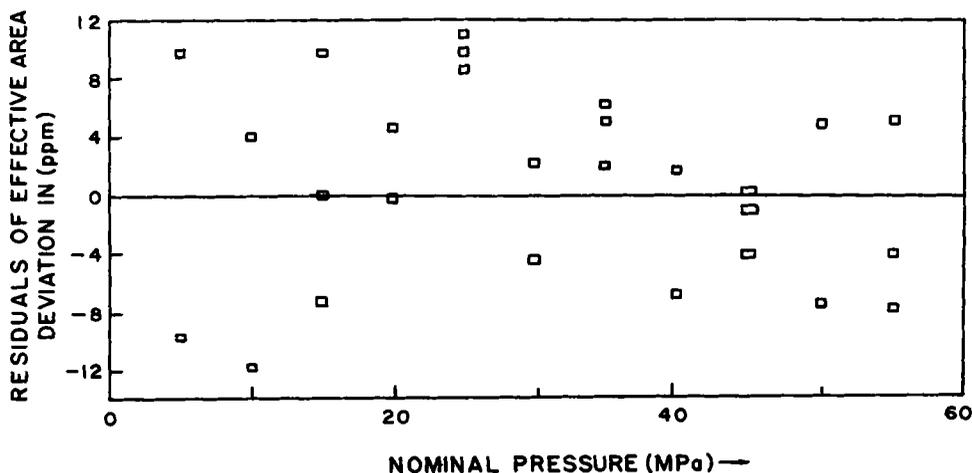
Figure 5. Deviation of measured values of the effective area of NPL-60 from the best linear fit  $A_e = 1.647127 \text{ E-5} (1 + 4.3 \text{ E-12} P)$  when calibrated by NPL-100.
