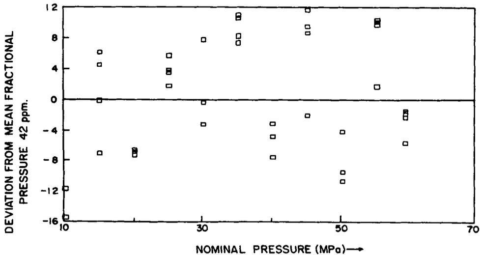
Figure 8. Fractional pressure differences from the mean value of 42 ppm between pressure measurements with the NPL-60 and NPL-140 pressure standard as a function of nominal applied pressure.
