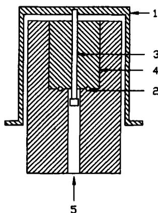
**Figure 1.** Schematic cross-sectional view of the piston and cylinder assembly for the pressure standard (NPL-60).
