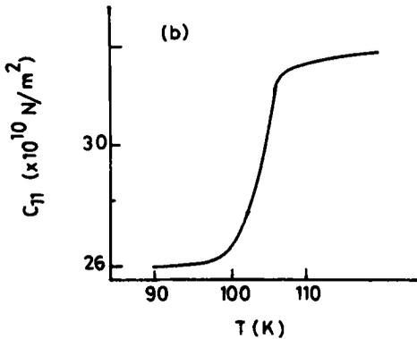
**Figure 1b.** Temperature variation of  $C_{11}$  near phase transition (experimental).
