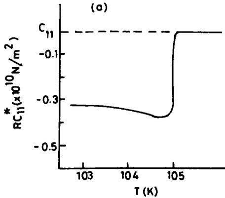
**Figure 1a.** Variation of the real part of  $C_{11}^*$  with respect to temperature close to the phase transition (theoretical).
