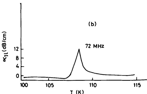
Figure 4b. Ultrasonic attenuation  $\alpha_{1l}$  of longitudinal wave as a function of temperature at high biaxial pressure (experimental).
