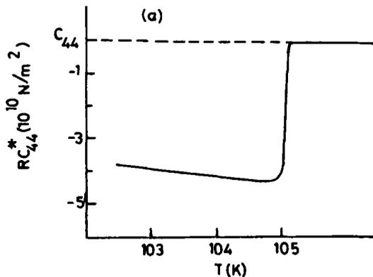
**Figure 2a.** Variation of the real part of  $C_{44}^*$  with respect to temperature close to the phase transition (theoretical).
