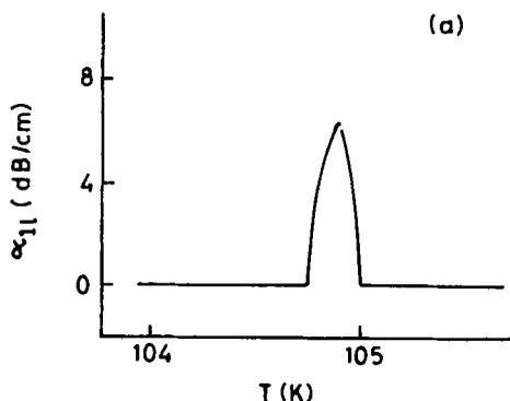
Figure 4a. Variation of attenuation of the longitudinal wave ( $\alpha_{1l}$ ) with respect to temperature close to the phase transition (theoretical).
