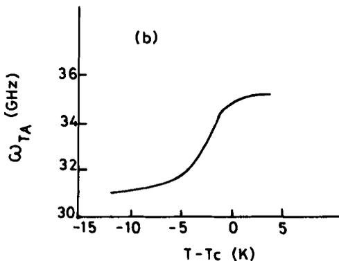
**Figure 2b.** Transverse acoustic mode  $\omega_{TA}$  frequency as a function of  $(T - T_c)$  (experimental).
