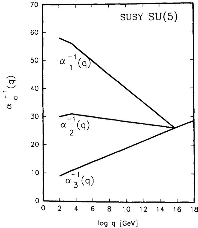
Figure 2. The evolution of the inverse coupling constants  $\alpha_{3C}^{-1}$ ,  $\alpha_{2L,R}^{-1}$ ,  $\alpha_{1(B-L)}^{-1}$  for the supersymmetric  $SU(5)$  GUT with  $M_{\text{susy}} \sim 1$  TeV.
