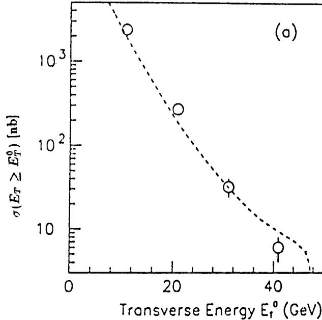
Figure 5. The total  $ep$  cross-section for transverse energies larger than  $E_T^0$  measured by ZEUS [20]. The curve is the HERWIG prediction, using the DG parametrization with  $p_{T,min} = 1.5$  GeV.
