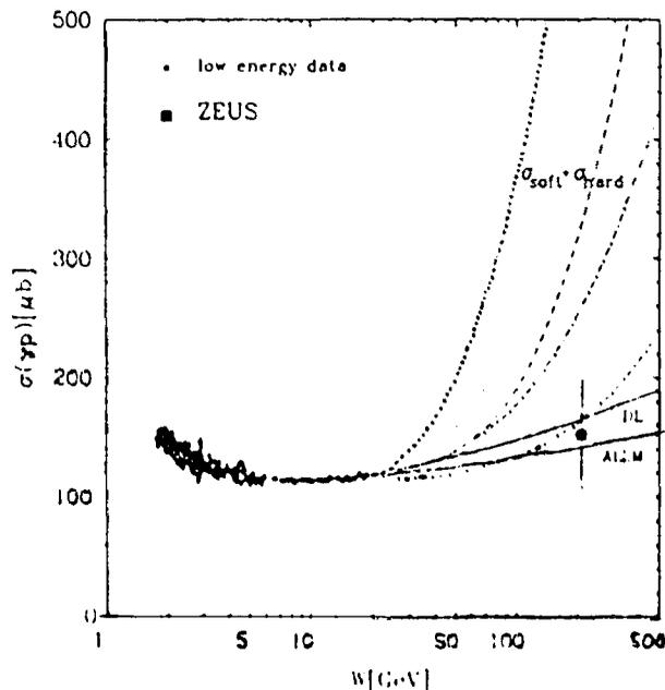
**Figure 8.** Comparison of low energy data and the recent ZEUS measurement of the total  $\gamma p$  cross-section with theoretical models. The two solid curves are Pomeron-based fits of the low energy data. The other curves are predictions of minijet models; the dot-dashed curves are for the DG parametrization, while the dotted and dashed curves are for LAC1. In both cases the upper (lower) curve is for  $p_{T,min} = 1.4$  (2.0) GeV. From ref.[24].
