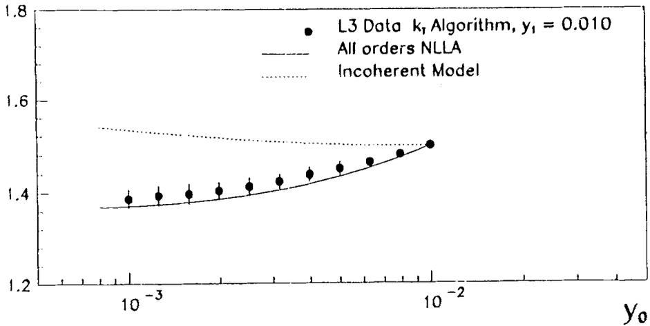
Figure 14. The three jet to two jet cluster multiplicity ratio as measured by L3.
