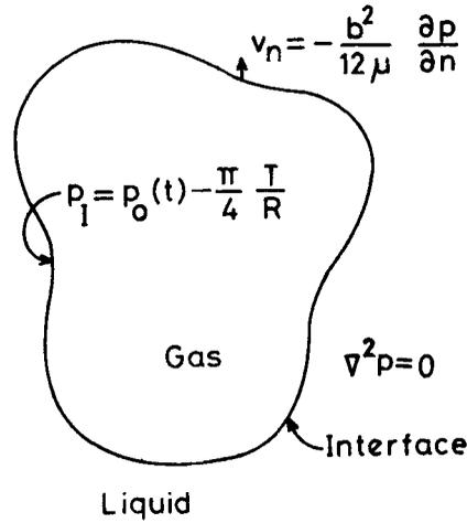
**Figure 1.** Schematic diagram of the experimental arrangement and the equations of motion.
