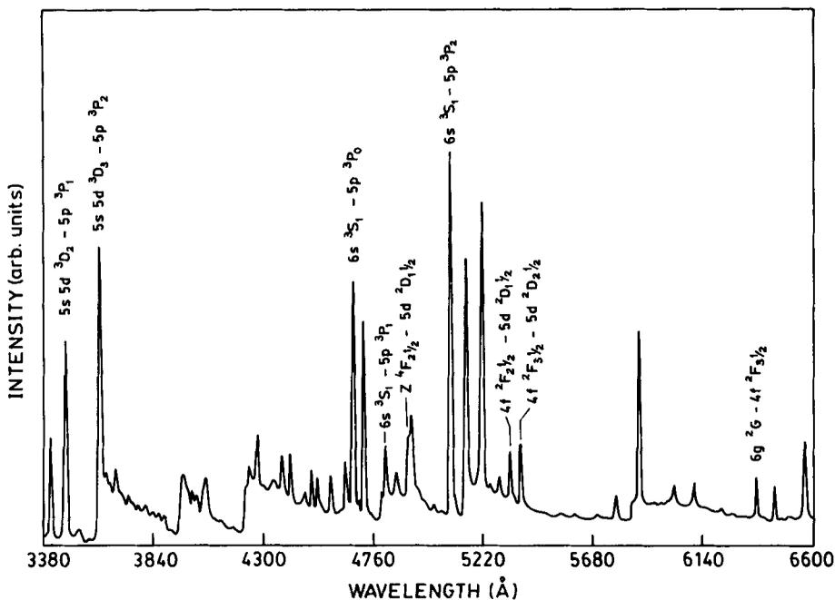
Figure 6. Visible spectrum of Cd metal vapor in the presence of tungsten plasma.
