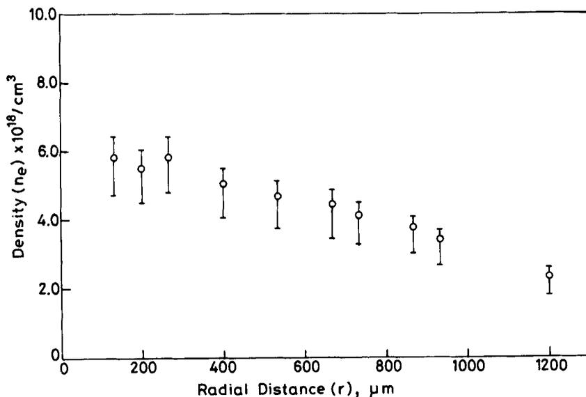
Figure 5. Radial density profile of tungsten plasma at 1–2 mm distance from the target.
