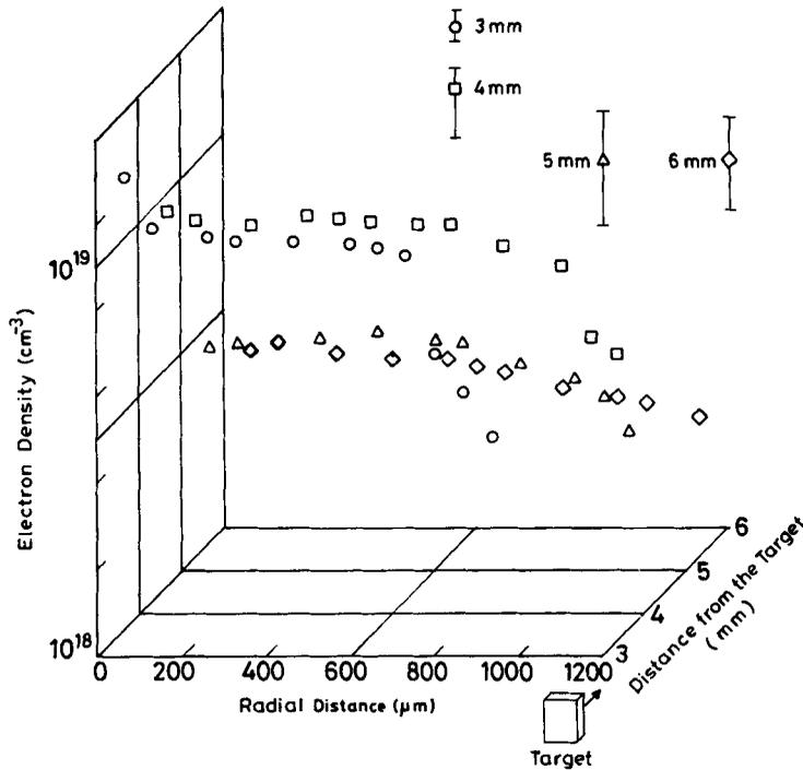
Figure 9. Radial density profiles of Cd plasma in the presence of tungsten target.
