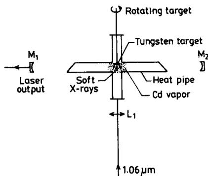
Figure 7. Experimental set-up for observing laser oscillations.
