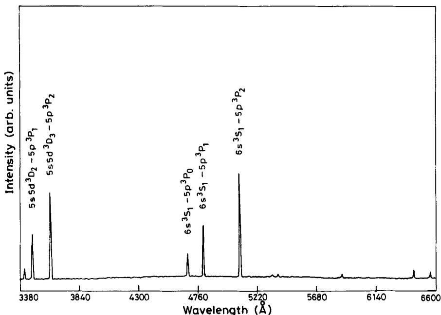
Figure 4. Visible spectrum of Cd metal vapor plasma at a He pressure of 77 torr.
