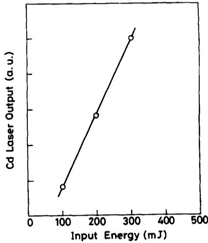
Figure 8. Variation of laser output with input laser ( $1.06 \mu\text{m}$ ) energy.
