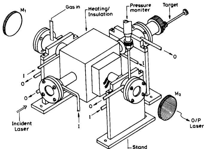
**Figure 1.** Design of crossed heat pipe.
