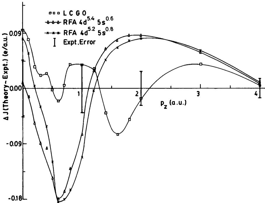
Figure 2. Difference ( $\Delta J$ ) profiles for bcc molybdenum. The theoretical result has been convoluted with the residual instrumental function (see text).
