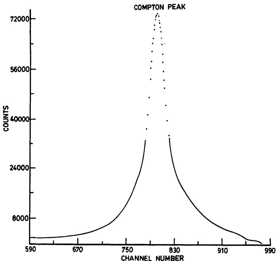
Figure 1. Raw experimental data for polycrystalline molybdenum. The elastic peak has been subtracted.
