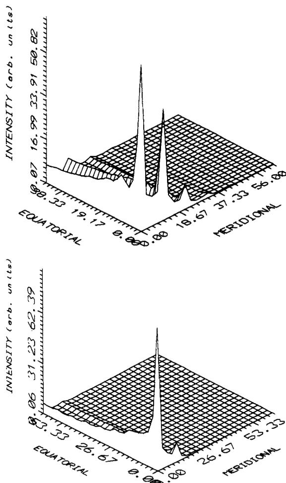
**Figure 3.** Iso-projection of X-ray diffraction pattern from a 3-D paracrystal for (a)  $g = 5\%$  and  $N = 5$  units (b)  $g = 15\%$  and  $N = 5$  units.
