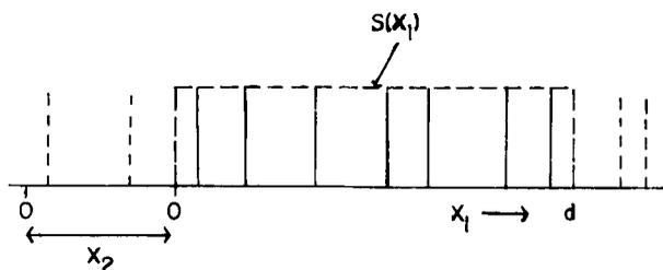
**Figure 1.** Electron density of a finite paracrystal. All delta functions outside the dotted shape amplitude are neglected. The quantity  $X_2$  allows different portions of the infinite lattice to fall within the shape amplitude.
