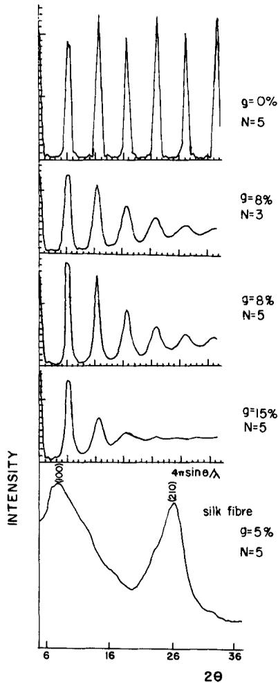
**Figure 2.** Intensity profiles of a 1-D paracrystal having various  $g$  (lattice distortion) and  $N$  (crystal units). Generated from the analytical expression including modification as mentioned in the text. XRD recording of a silk fibre is also given.
