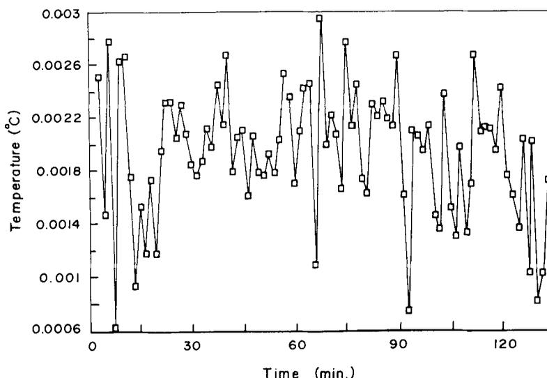
**Figure 3.** The fluctuations in the measured temperature with time—a systematic drift of about  $0.002^\circ\text{C}$  from the bath temperature is observed with a fluctuation of  $\pm 0.0005^\circ\text{C}$ .
