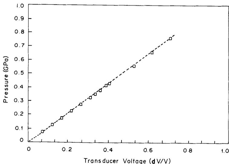
Figure 2. Pressure calibration of the strain gauge transducer—the relative output voltage is plotted with pressure.
