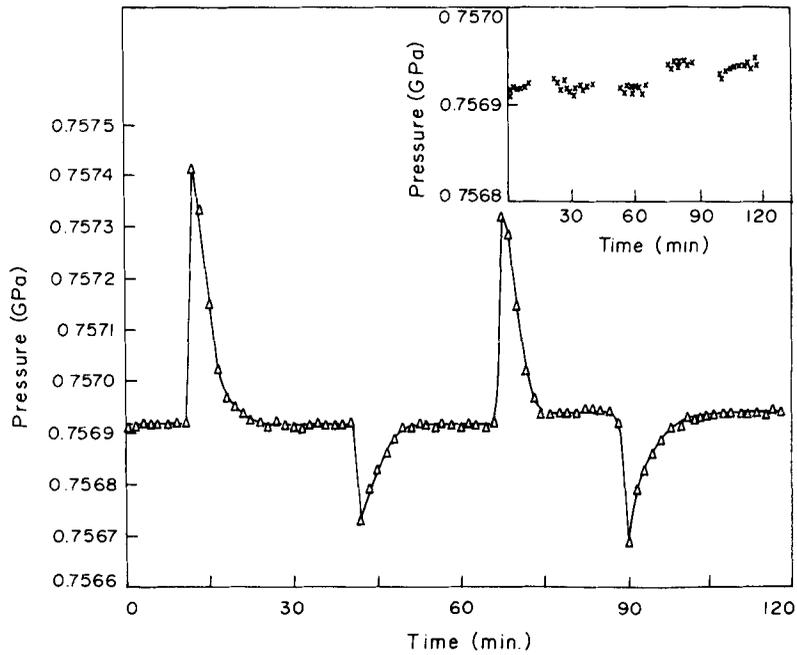
**Figure 4.** Readjustment of the liquid–solid phase equilibrium pressure at a temperature of 0.002°C after disturbance of the phase equilibrium by a sudden change in pressure. Inset shows pressure equilibrium points in the extended scale.
