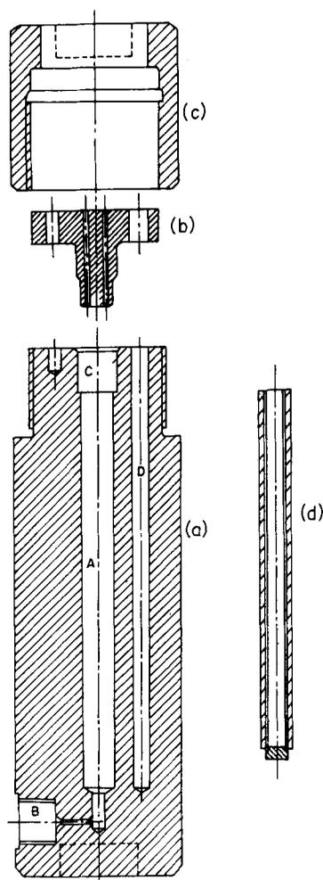
**Figure 1.** Schematic diagrams of different parts of the high pressure cell, a) container vessel—central cavity is for mounting the sample holder and side cavity is for mounting the PRT, b) Pressure holder cap, c) pressure retainer caps—pressure seal is obtained through the Bridgman seal which is formed by the combinations of different o-rings and placed at 45° angular portion of the cap and d) sample holder—stainless steel tube is press fitted inside a copper tube.
