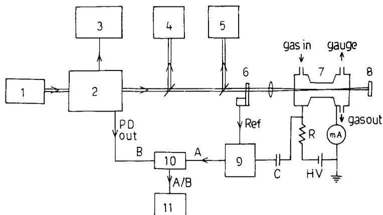
**Figure 1.** Experimental setup for high resolution OG spectroscopy. 1. Argon laser, 2. ring dye laser, 3. stabilock scanning electronics, 4. spectrum analyzer, 5. wavemeter, 6. chopper, 7. discharge cell, 8. beam stopper, 9. lock-in amp, 10. ratio meter, 11. chart recorder.
