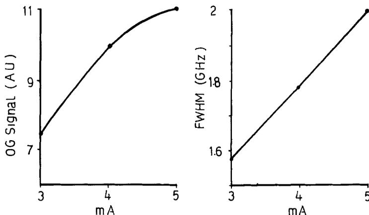
**Figure 4.** Variation of OG signal and fwhm at  $17388.7\text{ cm}^{-1}$  as a function of discharge current.
