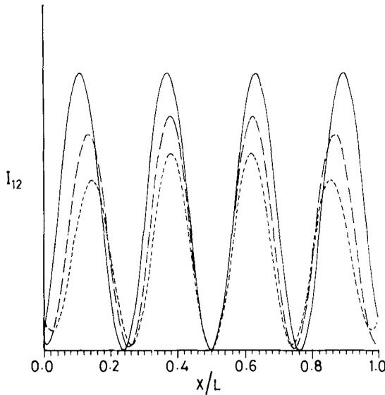
**Figure 2.** Plots of intensity  $I_{12}$  (in arbitrary units) versus relative position  $x/L$  at  $t=0$  for a dielectric scatterer satisfying condition (8) with  $|B|=0$  (—),  $|B|=1$  (— · —),  $|B|=2$  (----).
