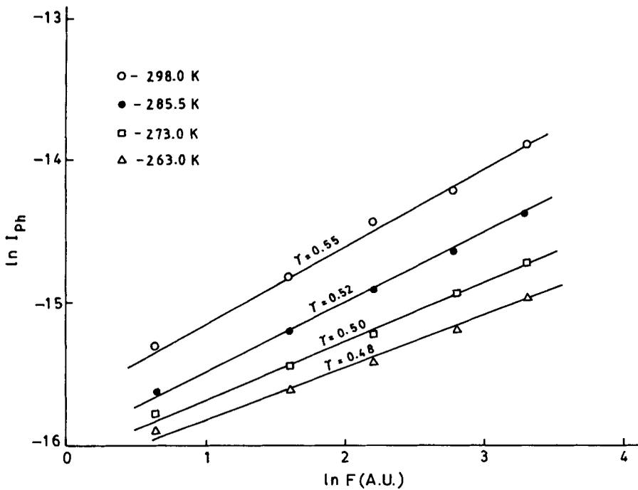
**Figure 5.** Variation of photocurrent with illumination level.
