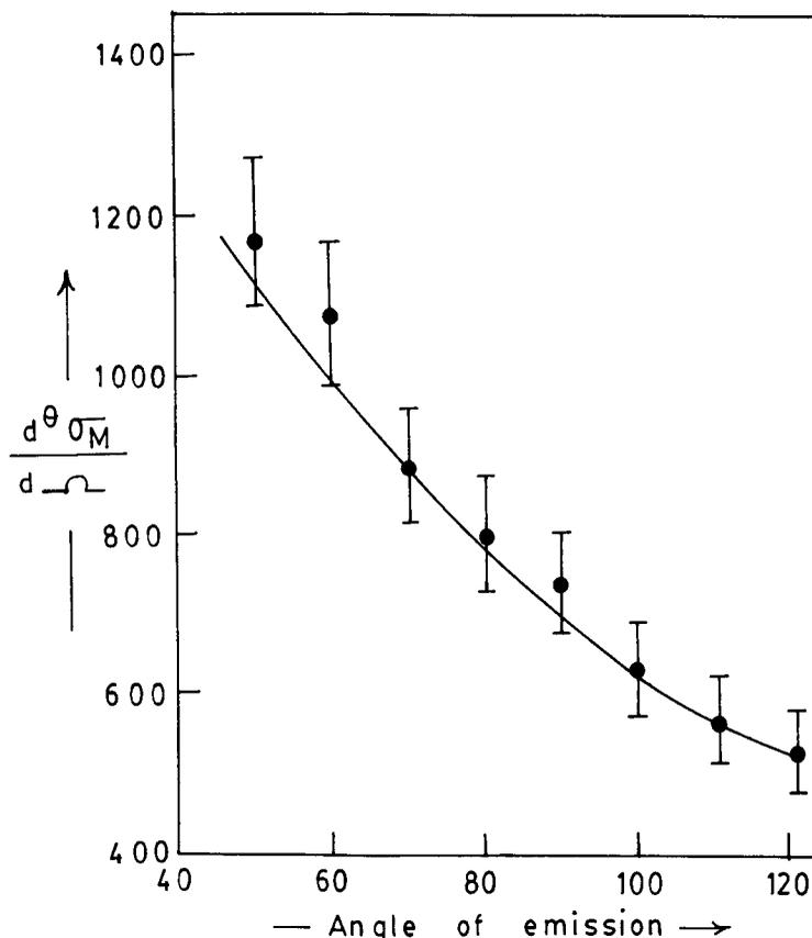
**Figure 2.** Variation of cross-sections  $d^\theta \sigma(M)/d\Omega$  of M shell fluorescent X-rays of Th with angle of emission  $\theta$ .  $\Phi$ , experimental points; full curve, fitted curve drawn with measured  $a_0$ ,  $a_1$  and  $a_2$  coefficients.
