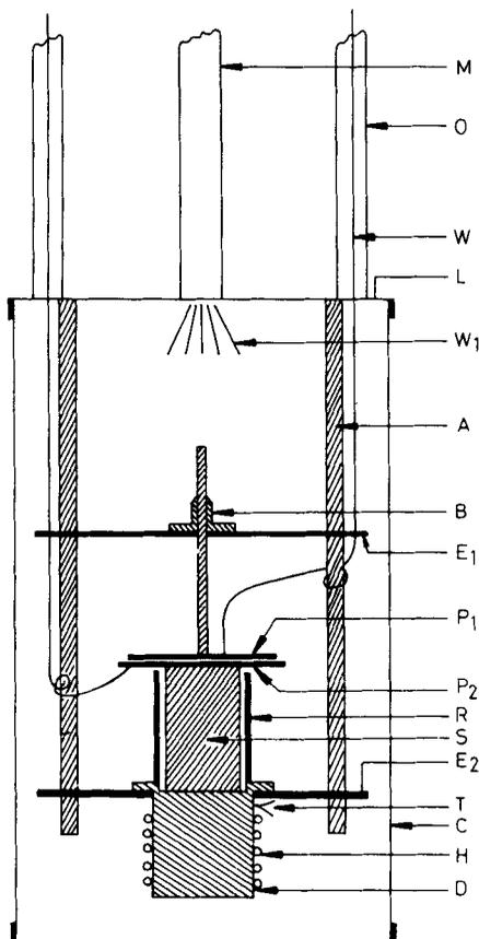
Figure 1. The dilatometer.
