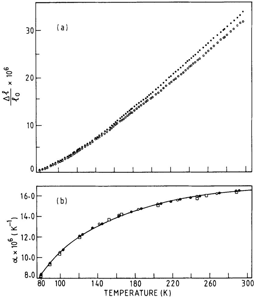
**Figure 2(a).** Temperature dependence of thermal strain  $\Delta l/l_0$ . ● Measured thermal strain; ○ after subtracting contribution due to expansion of condenser plate  $P_2$  (thickness 2 mm) and buckling of supports. (b) temperature dependence of the linear thermal coefficient of expansion of copper. — Present work; ○, Kroeger and Swenson (1977); ●, Rubin et al (1954); □, Hahn (1970).
