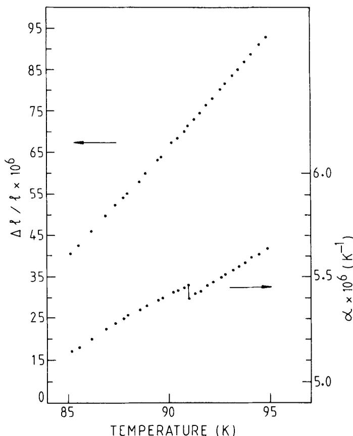
**Figure 3.** Thermal strain  $\Delta l/l_0$  and linear thermal coefficient,  $\alpha$ , of  $Y_1Ba_2Cu_3O_{6.9}$ , in the vicinity of superconducting critical temperature  $T_c$ .
