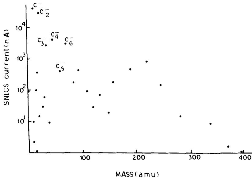
**Figure 2.** Negative ion current obtained from the SNICS source as a function of mass number.
