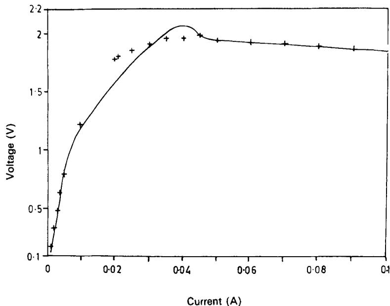
Figure 1. Current vs voltage characteristics of Qn-(TCNQ)<sub>2</sub> at 69 K (+ experimental; — theoretical).
