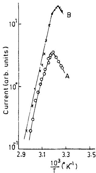
Figure 5. Arrhenius plots for dark current and photocurrent. A, dark current at IV; B, photocurrent at 9050 lux and at IV.
