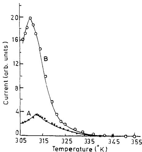
**Figure 4.** Variation of dark current and photocurrent with temperature. A, dark current at IV; B, photocurrent at 9050 lux and at IV.
