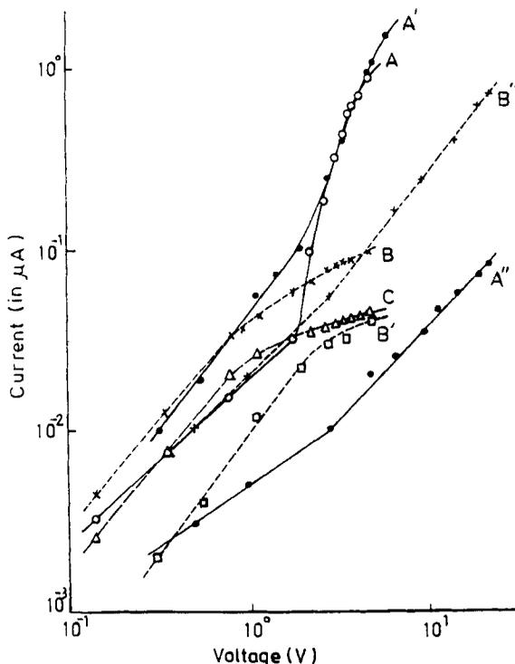
Figure 2. Variation of dark current and photocurrent with applied voltage. A, A' and A'', dark current for (20% MgO-80% ZnO), (50% MgO-50% ZnO) and 100% ZnO systems respectively; B, B' and B'', photocurrent at 4050 lux for (20% MgO-80% ZnO), (50% MgO-50% ZnO) and 100% ZnO systems respectively; C, photocurrent at 1200 lux for (20% MgO-80% ZnO) system. (Temperature = 22.5°C).
