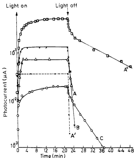
**Figure 6.** Rise and decay of photocurrent at different light intensities. A, A' and A'', at 4100 lux for (20% MgO-80% ZnO), (50% MgO-50% ZnO) and 100% ZnO systems respectively; C, at 110 lux for (20% MgO-80% ZnO) system; B at 9075 lux for (20% MgO-80% ZnO) system; (voltage = 4V and temperature = 17°C).
