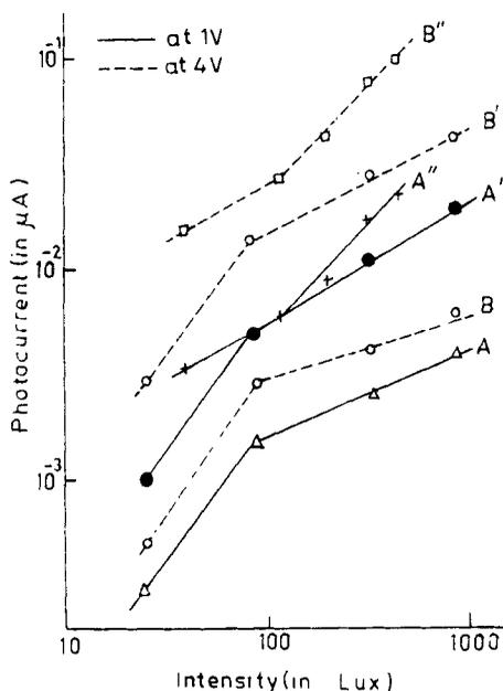
**Figure 3.** Variation of photocurrent with light intensity at different voltages. A, A' and A'', for (50% MgO–50% ZnO), (20% MgO–80% ZnO) and 100% ZnO samples respectively; B, B' and B'', for (20% MgO–80% ZnO), (50% MgO–50% ZnO) and 100% ZnO samples respectively (Temperature = 23°C).
