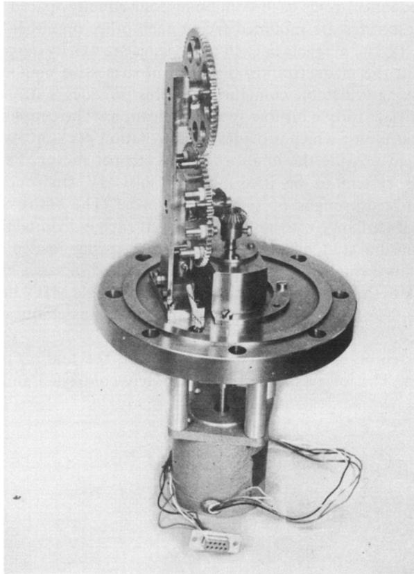
**Figure 3.** Side view of the assembly indicating the sensing studs and the spring loaded electrically isolated post.
