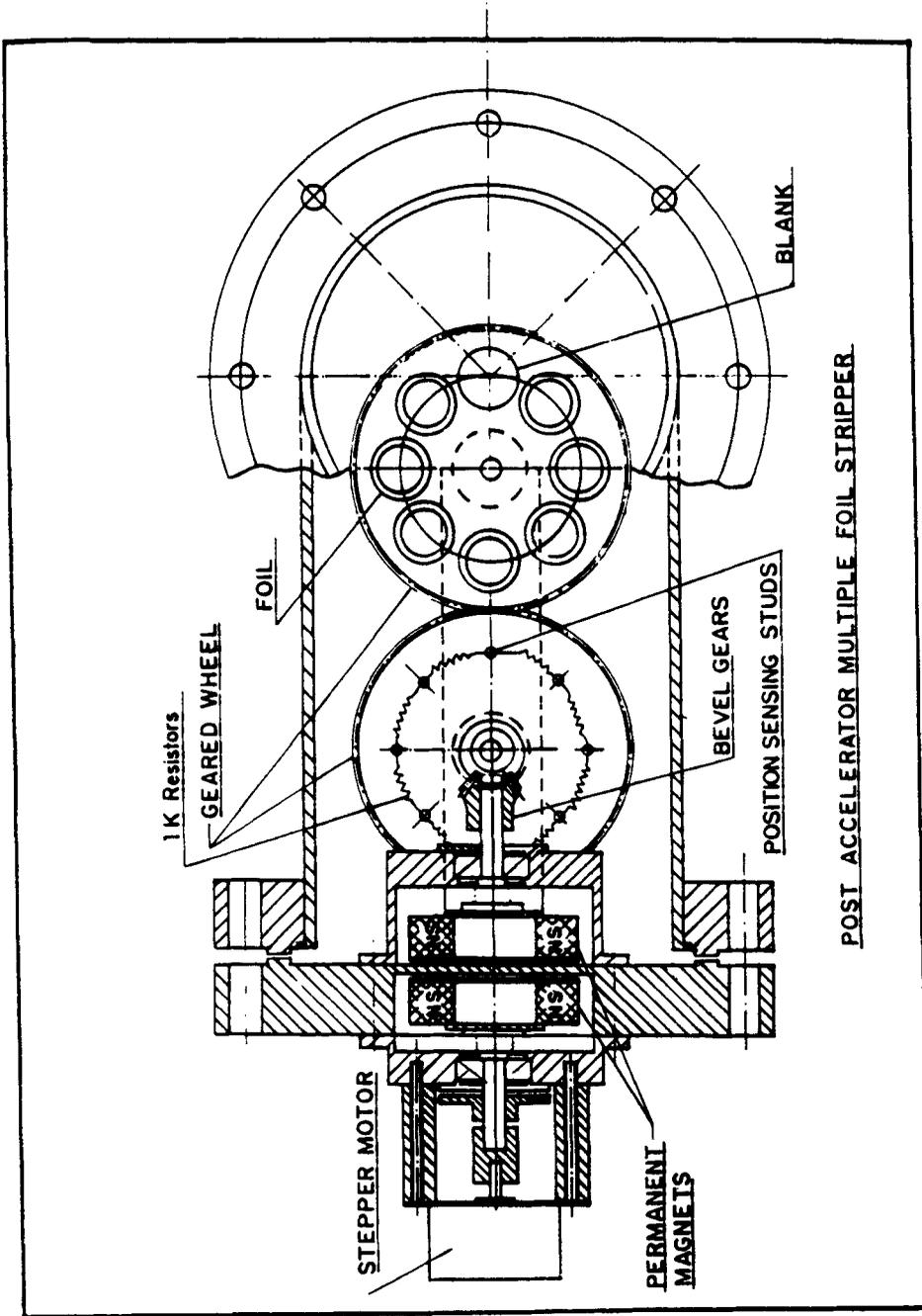
Figure 1. Assembly drawing of the multiple foil stripper.
