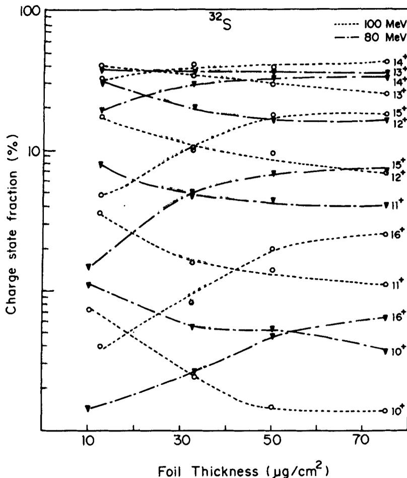
**Figure 4.** Normalized yields of  $^{32}\text{S}$  ions of different charge states measured on emergence from thin carbon foils of varying thicknesses. The incident beams were of 80 and 100 MeV with incident charge state of  $7^+$  and  $9^+$ , respectively.
