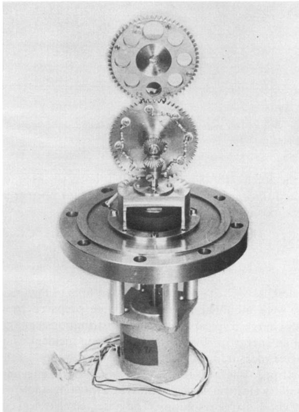
**Figure 2.** Front view of the stripper assembly showing the geared wheels, the resistance chain and one of the ceramic magnets. The larger size whole is used as blank for allowing the ion beam of original charge state produced in the machine.
