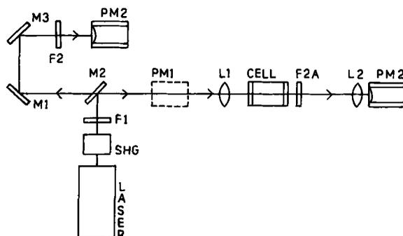
**Figure 1.** The experimental set up. SHG—Second harmonic generator, F1—Filter to cut  $1.06\ \mu\text{m}$  beam, PM1, PM2—Laser energy meters, F2—Laser line filter, F2A—Filter combination to cut scattered laser radiation and dye fluorescence, M2—Dichroic mirror to reflect pump beam and transmit the SRS beam, M1 and M3—Plane mirrors.
