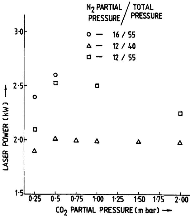
Figure 5. Effect of CO<sub>2</sub> partial pressure on laser power.
