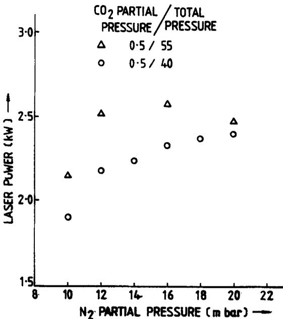
Figure 6. Effect of N<sub>2</sub> partial pressure on laser power.
