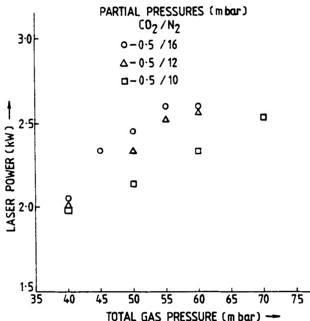
Figure 7. Effect of total gas pressure on laser power.
