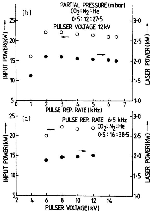
Figure 4. Effect of (a) pulser voltage and (b) its repetition rate on ultimate electrical input power and laser output power.
