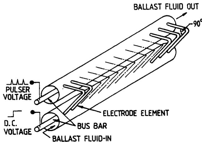
Figure 2. Schematic diagram of discharge electrode.
