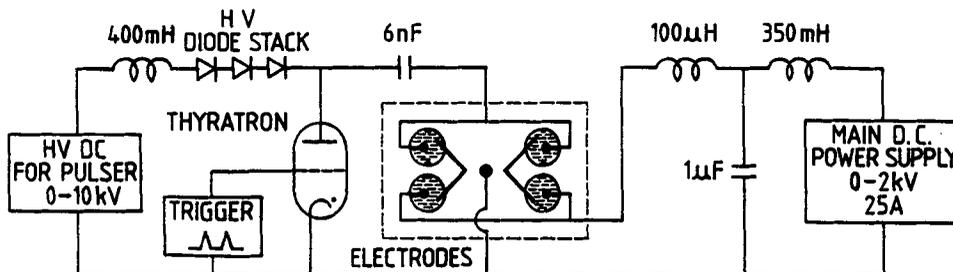
Figure 3. Electrical schematic of pulser and main discharge.
