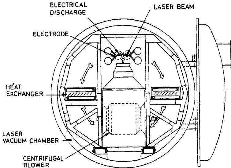
Figure 1. Schematic diagram of 2.5 kW transverse flow cw CO<sub>2</sub> laser.
