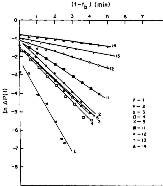
Figure 2.  $\ln P(t)$  versus  $(t - t_b)$  plot at the various percentages of liquid phase.
