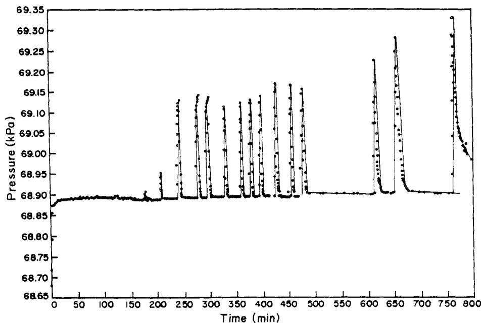
Figure 1. Observations of argon triple point pressure at various percentages of liquid phase.
