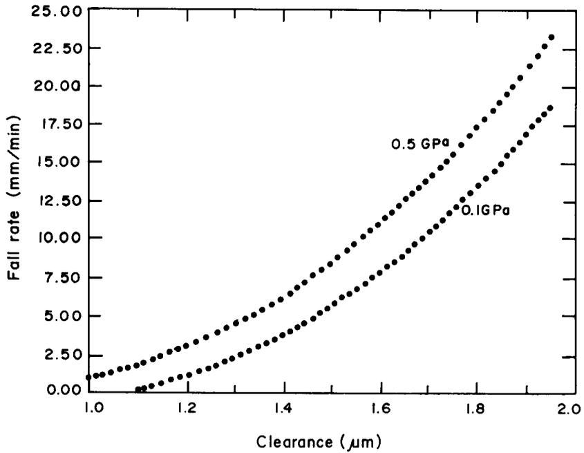
Figure 3. Computed fall rate versus initial clearance curve at two different pressures.
