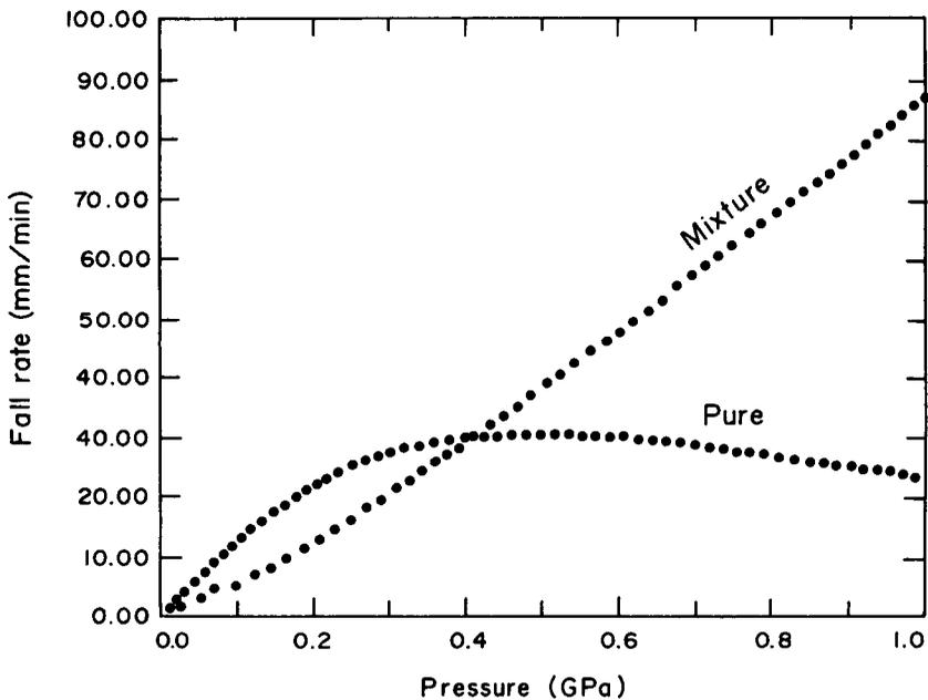
Figure 4. Computed fall rate versus pressure curve for both the pure fluid and the mixture.
