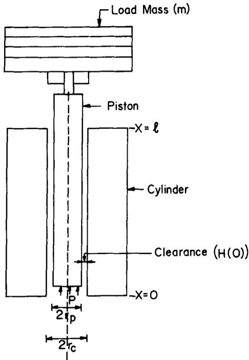
Figure 1. Schematic diagram of a simple piston cylinder assembly.
