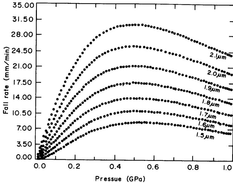
Figure 2. Computed fall rate versus pressure curve at different initial clearances.
