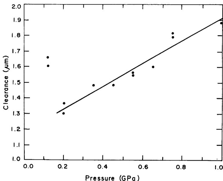
Figure 5. Initial clearance computed from the experimentally obtained fall rate data, is shown as a function of pressure.
