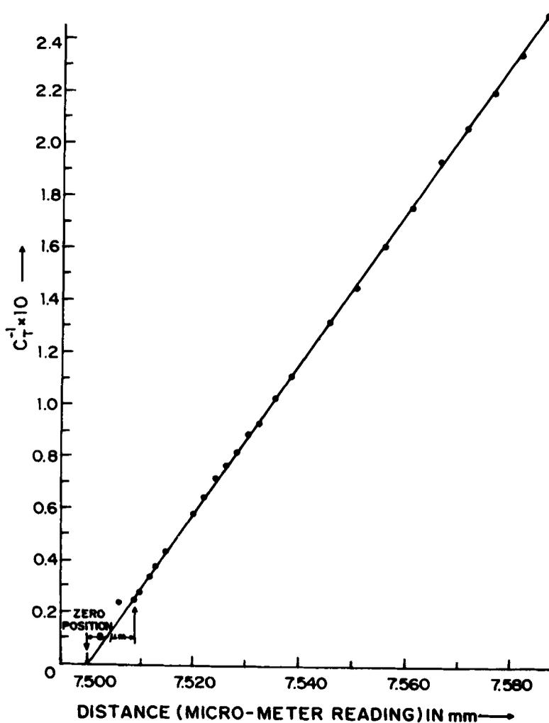
Figure 6. The inverse of capacitance ( $C_T^{-1}$ ) between the target and stopper foils measured as a function of the micrometer position ( $d$ ).
