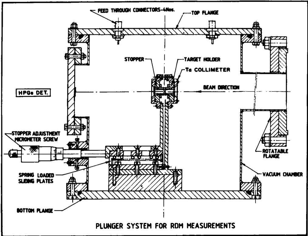
Figure 4. Schematic diagram of the plunger assembly inside the vacuum chamber.
