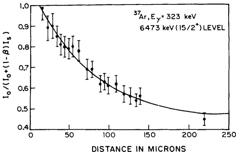
Figure 8. The plot of  $I_0/(I_0 + (1 - \beta)I_s)$  vs  $D$  for the 323 keV  $\gamma$ -ray deexciting 6473 keV level in  $^{37}\text{Ar}$ .
