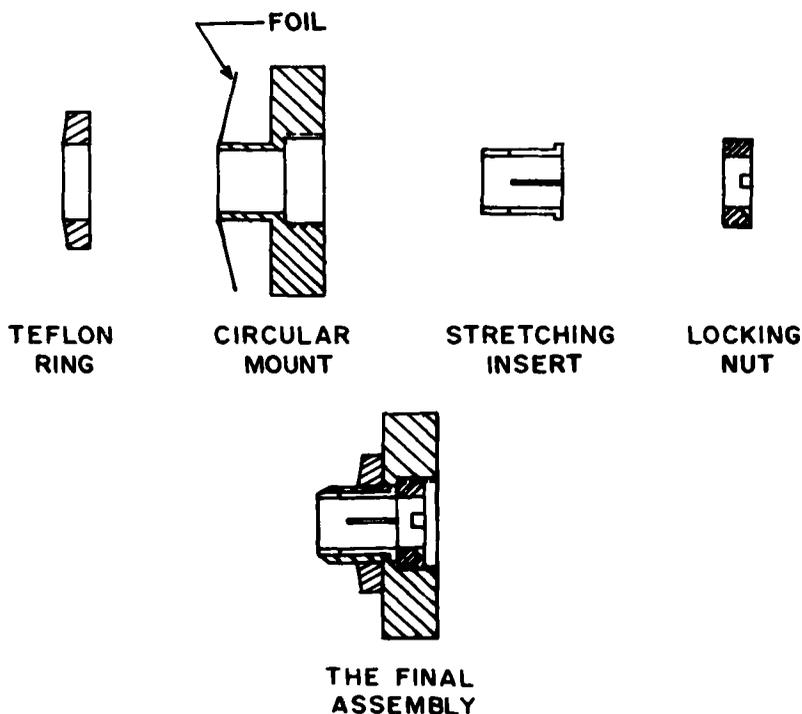
**Figure 1.** The components and assembly of the target holder used for stretching of tantalum foils.
