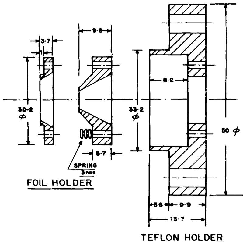
**Figure 2.** The target holder used for stretching thin (1 to 2 mg/cm<sup>2</sup> thickness) tantalum foils. The dimensions indicated are in mm.
