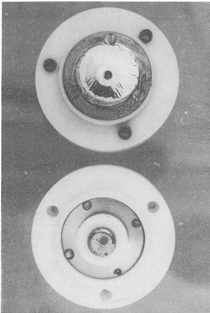
Figure 3. The photograph of the stretched target and stopper foils used in the present experiment.
