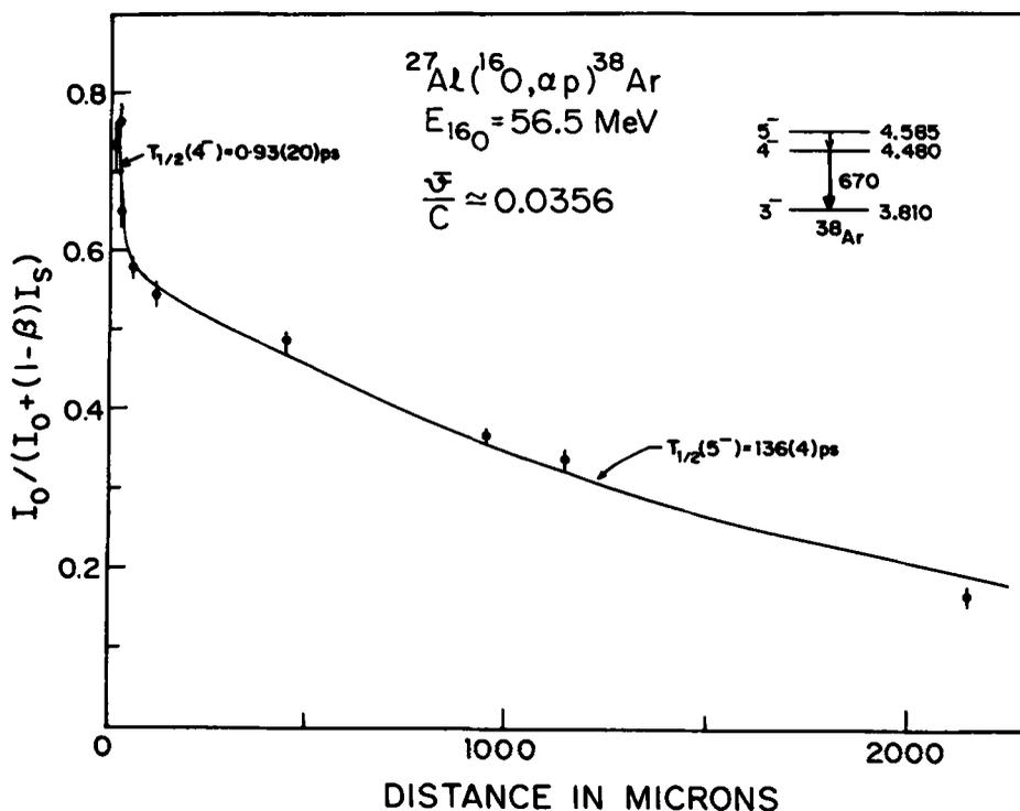
Figure 9. The plot of  $I_0/(I_0 + (1 - \beta)I_s)$  vs  $D$  for the 670 keV  $\gamma$ -ray deexciting the 4480 keV level in  $^{38}\text{Ar}$ . The measurement gave a value of  $T_{1/2} = 136(4)$  ps for the 4585 keV level and  $T_{1/2} = 0.93(20)$  ps for the 4480 keV level in  $^{38}\text{Ar}$ .
