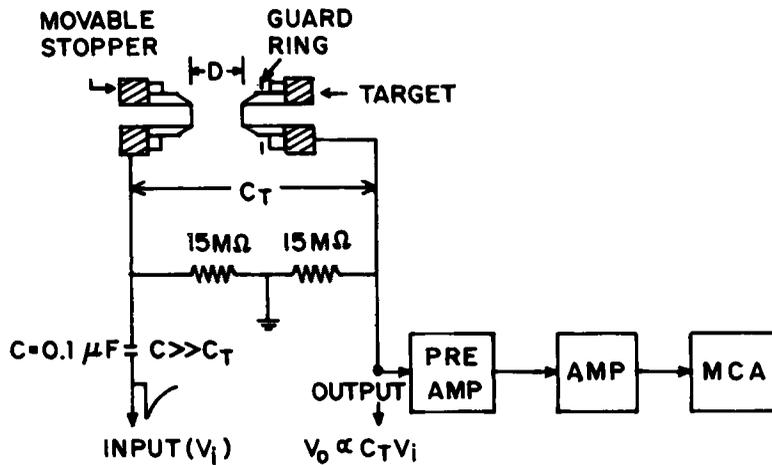
Figure 5. Schematic diagram for the arrangement used for monitoring the target to stopper distance through the capacitance measurement technique.
