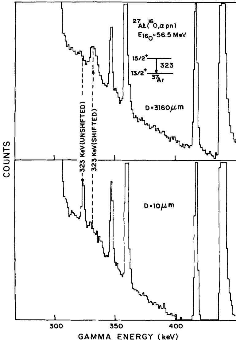
**Figure 7.** A partial  $\gamma$ -ray spectrum showing 323 keV  $\gamma$ -ray deexciting 6474 keV ( $15/2^+$ ) state in  ${}^{37}\text{Ar}$  produced in  ${}^{27}\text{Al}({}^{16}\text{O}, \alpha pn)$  reaction at  $E_{{}^{16}\text{O}} \sim 56.5$  MeV. The spectrum at the bottom was obtained for a target to stopper distance  $D = 10 \mu\text{m}$  showing unshifted 323 keV  $\gamma$ -ray. The spectrum at top is for  $D = 3160 \mu\text{m}$  showing the fully shifted 323 keV  $\gamma$ -ray.
