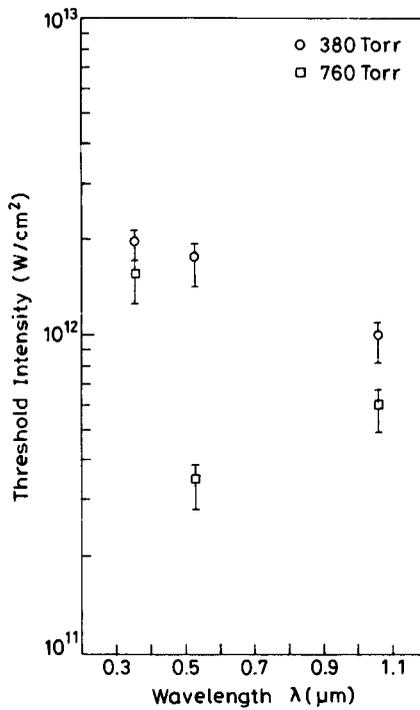
**Figure 2.** Dependence of breakdown threshold intensity on wavelength of radiation for two pressures.
