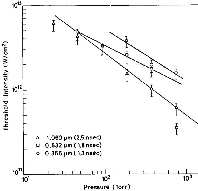
**Figure 1.** Dependence of breakdown threshold intensity on pressure of air. The pulse widths of various wavelengths used are shown in parantheses.
