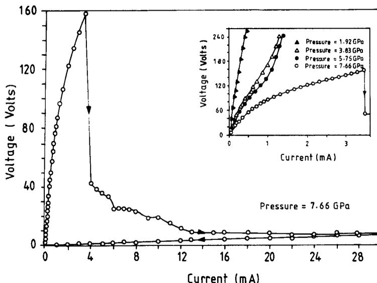
Figure 2. Current-voltage characteristics of *o*-tolidine-DDQ at different pressures, temperature = 300 K.
