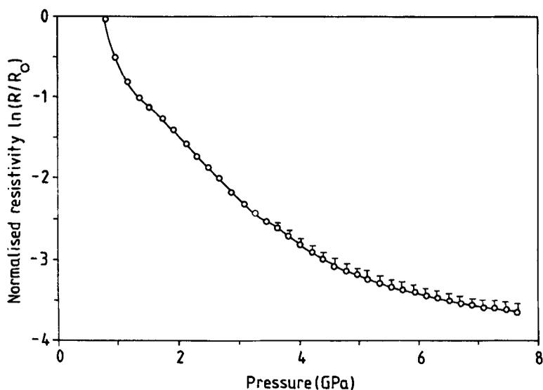
Figure 1. Pressure dependence of normalized resistivity of *o*-tolidine-DDQ,  $T = 300 \text{ K}$ .
