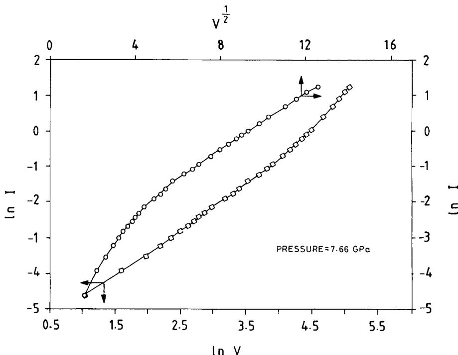
Figure 3. Plot of  $\ln I$  vs.  $\ln V$  and  $\ln I$  vs.  $V^{1/2}$  of *o*-tolidine-DDQ at a pressure of 7.66 GPa.
