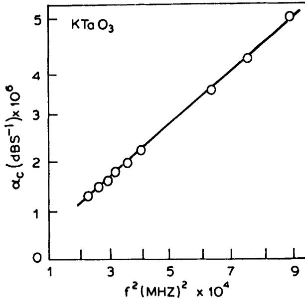
Figure 3. Critical attenuation as a function of  $f^2$  at  $\Delta T = 10$  K above  $T_c$ .
