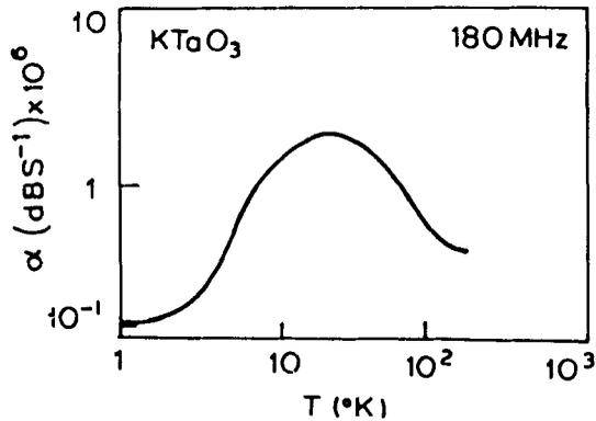
Figure 1. Ultrasonic attenuation of longitudinal wave propagating along (100) direction vs temperature.
