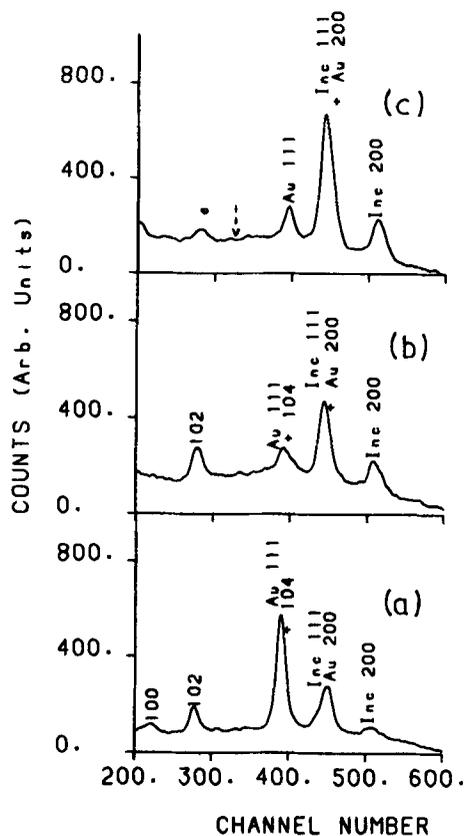
**Figure 1.** EDXRD pattern of  $AlPO_4$  (a)  $\sim 0.1$  GPa (b) 2.5 GPa (c) 14 GPa.
