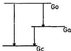
**Figure 2.** The three-level energy diagram which explains the pressure-induced crystal-to-amorphous transition. The kinetic conditions require  $\tau_{0 \rightarrow a} \ll \tau_{0 \rightarrow c}$  and  $\tau_{0 \rightarrow a} \ll \tau_{a \rightarrow c}$ .
