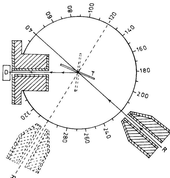
**Figure 1.** Experimental set up used for the investigation of angular distribution of L shell fluorescent X-rays. R-radioactive source ( $^{241}\text{Am}$ ), T-target, D-detector Si(Li).
