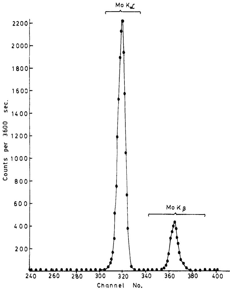
Figure 4. Spectrum of Mo K X-rays recorded with Si(Li) X-ray spectrometer at emission angle of 90°.
