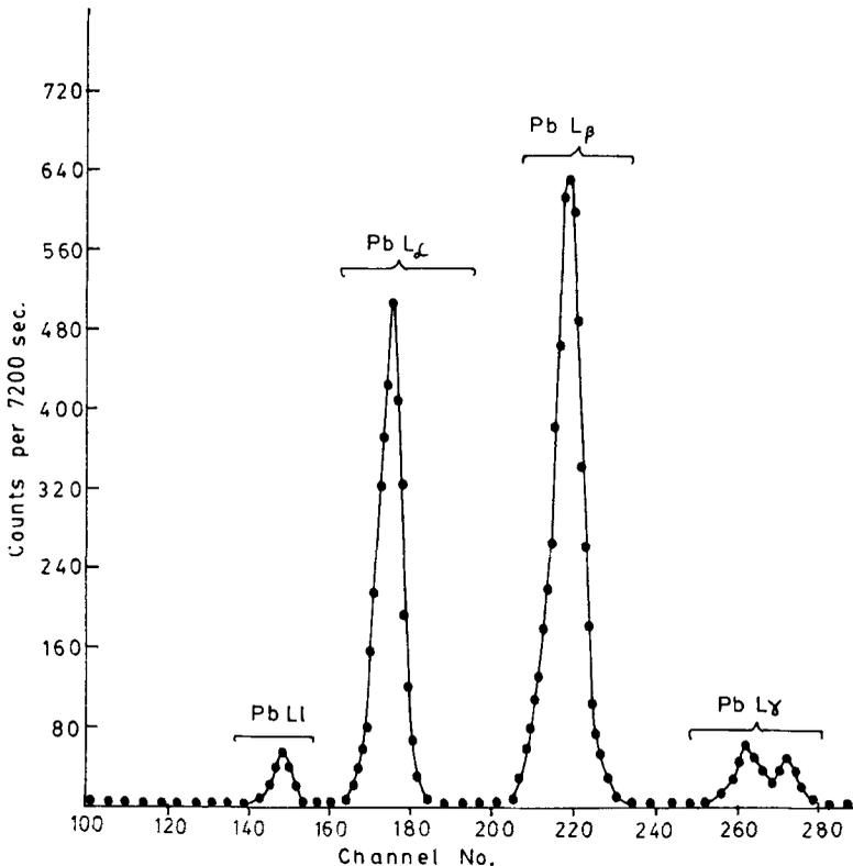
**Figure 2.** Spectrum of Pb L X-rays recorded with Si(Li) X-ray spectrometer at emission angle of  $90^\circ$ .
