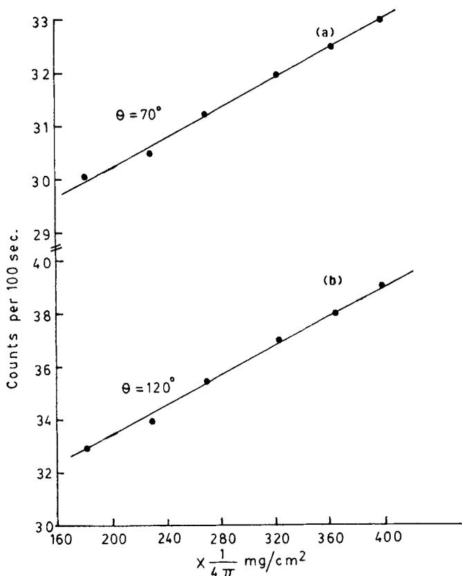
**Figure 3.** Variation of number of counts under  $L_\beta$  X-ray peak of lead targets against the thickness of targets at emission angles of  $70^\circ$  and  $120^\circ$ .
