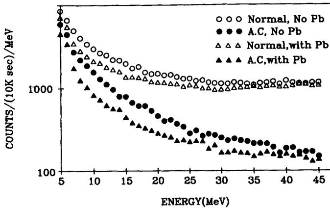
Figure 9. Cosmic ray background spectra measured in the NaI(Tl) detector array. Spectra with different conditions of active and passive shielding are shown.
