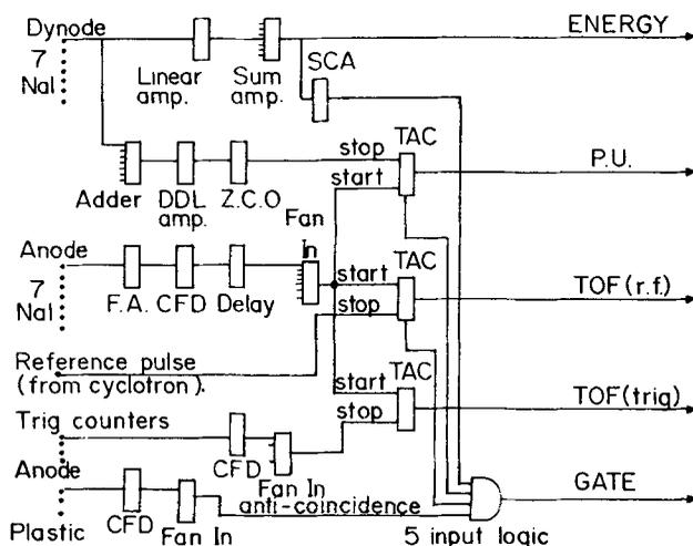
**Figure 2.** Block diagram of the electronics; at VECC, the data acquisition system based on NORD computer was used to collect four parameter list mode data, in coincidence with the 'GATE'.
