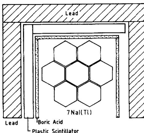
**Figure 1.** Schematic diagram of the front view of the set up; The NaI(Tl) detector array is surrounded by boric acid and 3 plastic scintillators which are placed on the side, top and front (not shown in figure). Lead bricks are placed on the side and the top.
