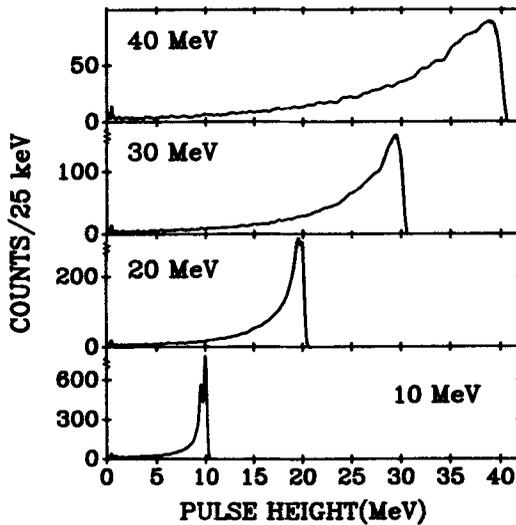
Figure 11. Calculated response of the 7 NaI(Tl) detector array to monochromatic  $\gamma$ -rays of different energies. The full energy peak and the escape peaks can be recognized. The fluctuations in the spectra are because of finite number of events run in the Monte Carlo simulation program.
