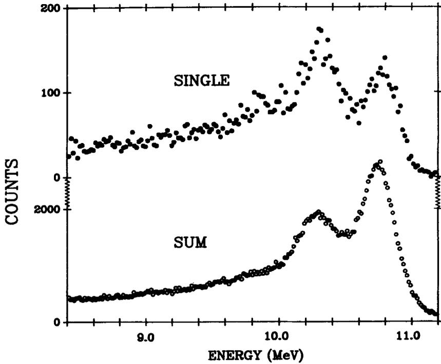
Figure 10. Measured line shapes for the 10.76 MeV  $\gamma$ -ray produced in the  $^{27}\text{Al}(p, \gamma)^{28}\text{Si}$  reaction, single detector alone, and for all the detectors summed together.
