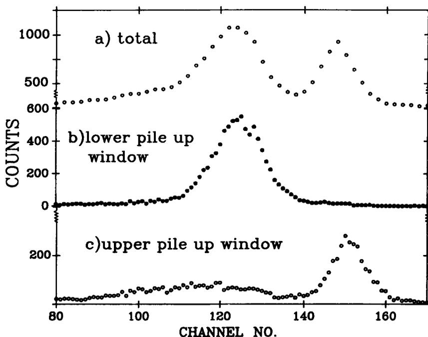
**Figure 8.** TOF(r.f.) spectra for energy window 15–20 MeV. **a)** Inclusive TOF(r.f.) spectrum; **b)** The spectrum in **a)** gated by a lower pile up window (channel # 160–186) in the pile up TAC spectrum (see figure 7); **c)** The spectrum in **a)** gated by an upper pile up window (channel # 187–200) in the pile up TAC spectrum (see figure 7).
