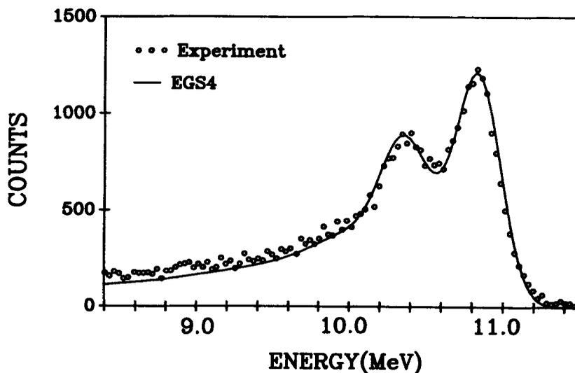
Figure 12. Calculated and measured response of the detector array to 10.76 MeV  $\gamma$ -ray in the  $^{27}\text{Al}(p, \gamma)^{28}\text{Si}$  reaction.
