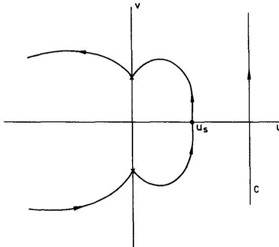
**Figure 1(a).** The steepest descent contour for the ground-state wave function of FRW model in  $Ha < 1$ . Near the saddle point  $k = (H/3) \tan \alpha$  on the real axis of  $k$ -plane, the path is the straight line  $u = (H/3) \tan \alpha$ . The contour also passes through the branch points  $k = \pm i$ , located by crosses.
