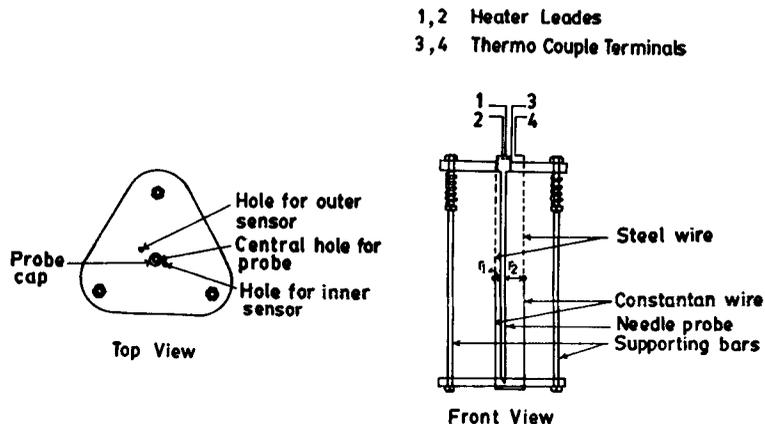
Figure 1. Design of differential temperature sensors probe.
