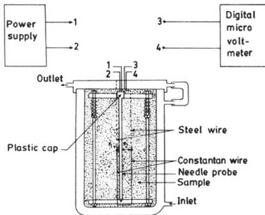
Figure 2. Experimental arrangement for conductivity and diffusivity determination.
