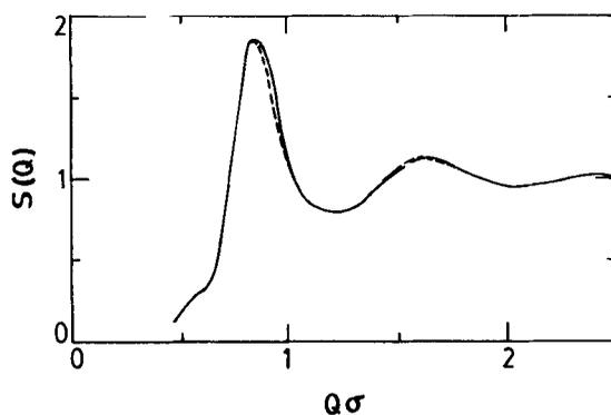
**Figure 3.** Comparison of structure factors  $S(Q)$  vs  $Q$  (in units of  $\sigma^{-1}$ ) calculated from MC (—) and BD (---) for Sogami potentials with  $n_i = 1.75 \times 10^{15} \text{ cm}^{-3}$ ,  $n_p$  and  $Z$  as in figure 1.
