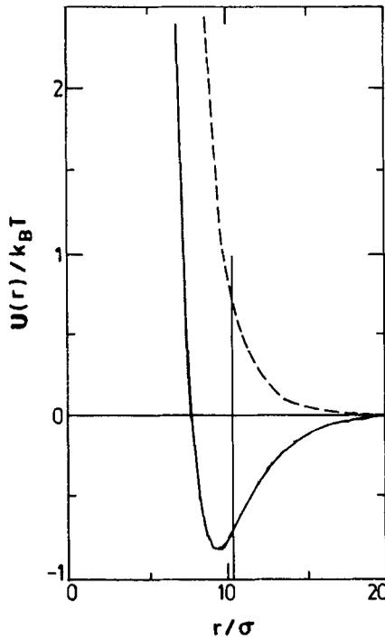
Figure 1. Pair potential  $U(r)$  in units of  $k_B T$  vs distance of separation  $r$  in units of  $\sigma$ . Continuous line is Sogami potential for  $\sigma = 0.109 \mu\text{m}$ ,  $n_p = 1.33 \times 10^{12} \text{cm}^{-3}$ ,  $Z = 600$  with  $n_i = 1.75 \times 10^{15} \text{cm}^{-3}$  and dotted line is Yukawa potential for  $n_i = 2.1 \times 10^{15} \text{cm}^{-3}$  with  $n_p$  and  $Z$  same as above. The vertical line is at interparticle separation  $2a_s = 10.35\sigma$ .
