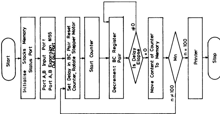
Figure 4. Flowchart explaining the operation of the processor.
