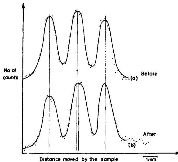
**Figure 6.** A plot of number of counts versus distance. Dots represent the print out of the radioactive concentration profile from the autoscanner a) Before electromigration. b) Annealed at 473 K. The current density is  $2.1 \times 10^8\ \text{A/m}^2$ . The continuous line is the best fit to the experimental dots.
