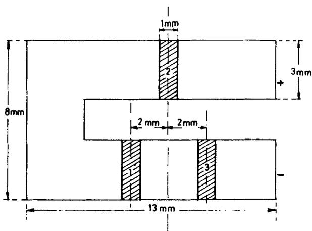
Figure 1. The experimental sample consisting of  $U$  shaped tin thin film and the three radioactive dots.
