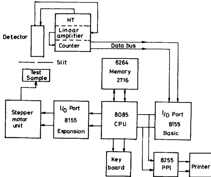
Figure 3. Block diagram explaining the signal processing from the test sample to the printer.
