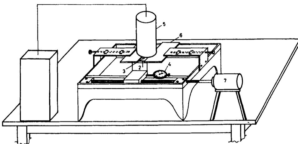
Figure 2. Experimental testing jig for mounting the sample and scanning the radioactivity. 1. Single channel analyser, 2. Sample holder, 3. Sample, 4. Dial gauge, 5. Detector, 6. Adjustable slit, 7. Stepper motor.
