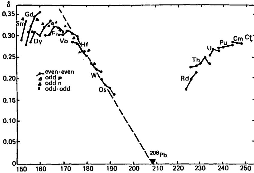
Figure 3. Quadrupole deformations of heavy nuclei. The broken line is drawn with slope given by expression (11) corresponding to rhomboid-shaped orbits in the axis-of-symmetry plane. The actinide region is too narrow for comparison (see also figure 2).
