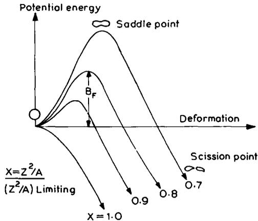
Figure 2. Potential energy vs deformation for increasing  $Z^2/A$ .
