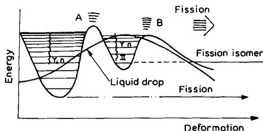
Figure 4. A schematic diagram of double-humped fission barrier.
