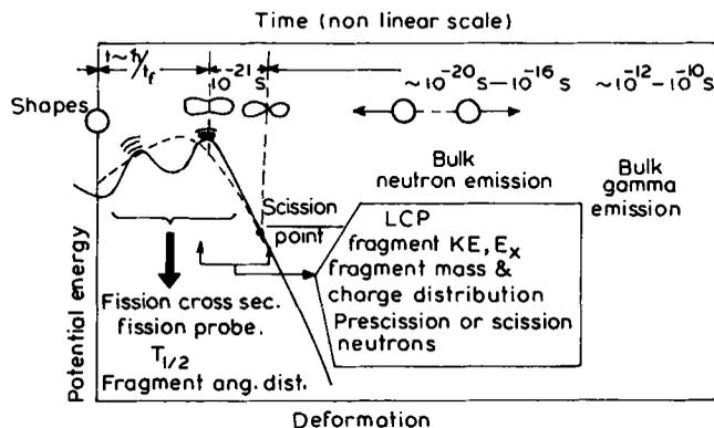
Figure 3. Different stages of the fission process and the corresponding time scales.
