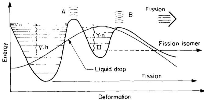
Figure 3. Schematic diagram of double-humped fission barrier.
