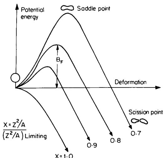
**Figure 2.** A schematic representation of the potential energy versus deformation for increasing values of  $Z^2/A$ .
