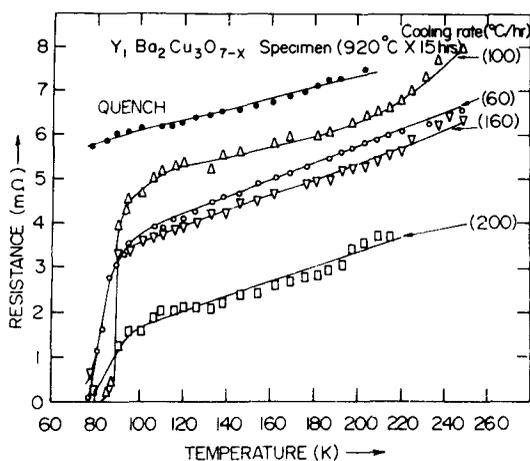
**Figure 1** Resistance versus temperature plots of the  $\text{Y}_1\text{Ba}_2\text{Cu}_3\text{O}_{7-x}$  specimens sintered  $920^\circ\text{C} \times 15\text{h}$  and cooled at a rate of 60, 100, 160, 200  $^\circ\text{C/h}$  and quenched to 77 K
