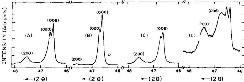
Figure 3 X-ray diffraction peaks between  $2\theta = 46-48^\circ$  for  $Y_1Ba_2Cu_3O_{7-x}$  specimens cooled at 60°C/h (A), 100°C/h (B), 200°C/h (C), and quenched to 77 K (D)
