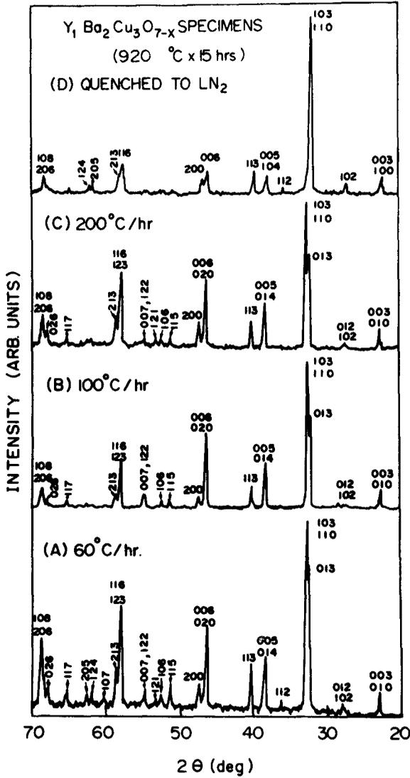
Figure 2 Room temperature diffraction spectra of the specimens cooled at the rate of 60, 100, 200°C/h (A-C) and quenched to 77K (D)
