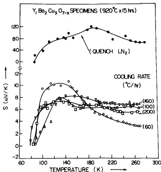
**Figure 4** Measured thermopower corrected for the thermopower of pure copper leads, plotted against temperature for  $Y_1Ba_2Cu_3O_{7-x}$  specimens as listed in table 1. All values are positive. The quenched sample has a very large thermopower.
