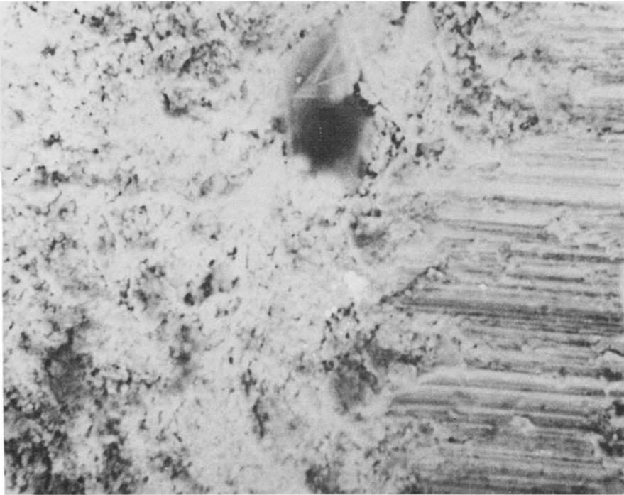
**Figure 4.** Microphotograph of cross-section of copper tube and superconductor solid monolith ( $\times 1000$ ) obtained by compaction.
