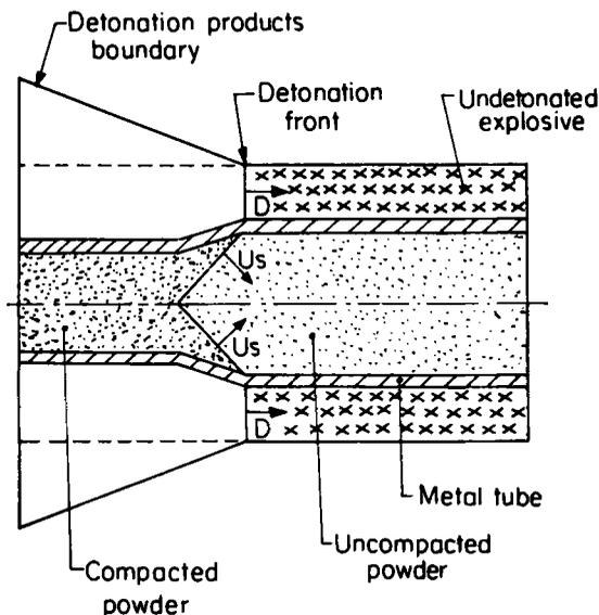
**Figure 1.** Compaction of powder in a cylindrical tube by axisymmetrical (conical) shock wave.
