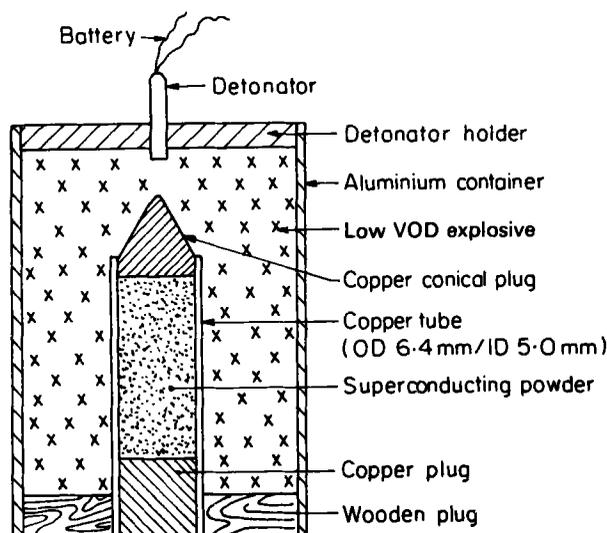
Figure 2. Explosive compaction of superconducting powder.
