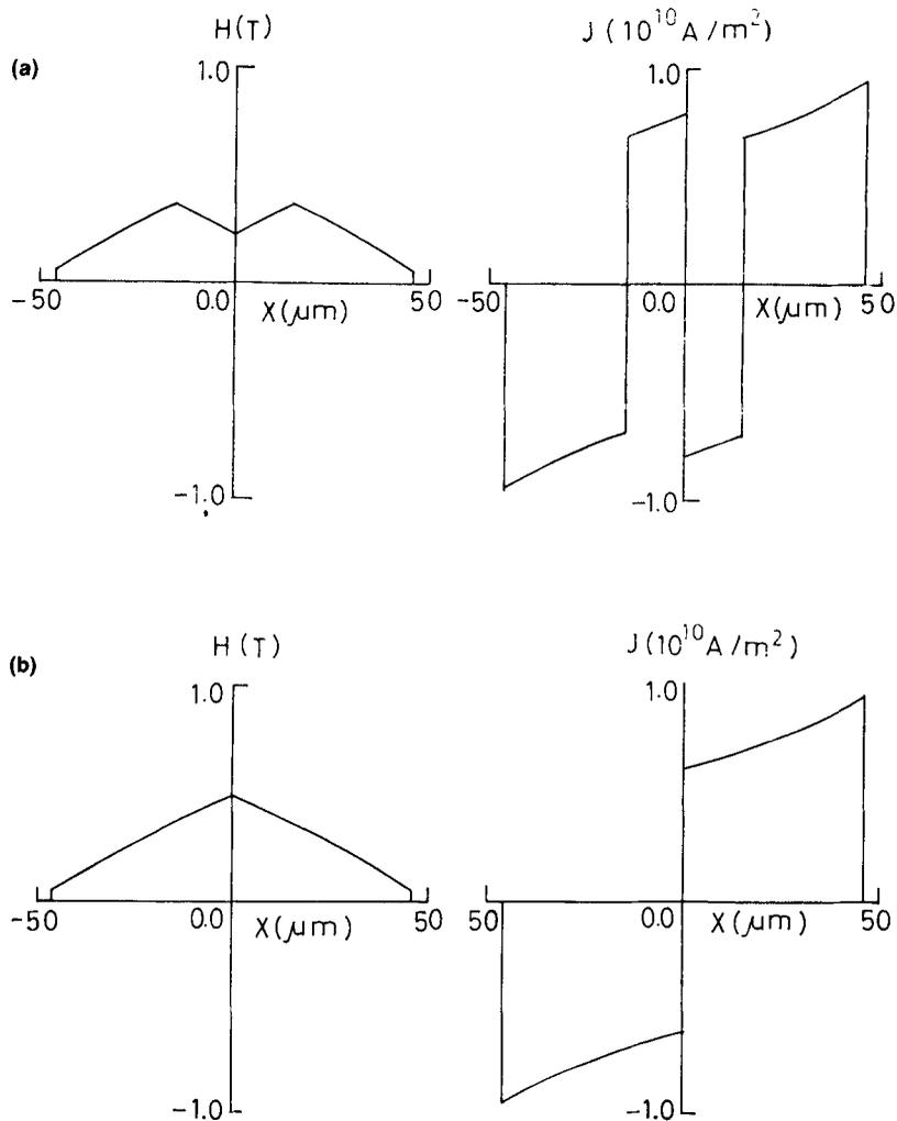
**Figure 3.** Magnetic field profile and the current density distribution inside the slab when the external field is reversed to zero from (a)  $H_{\max} = 0.63$  tesla and (b)  $H_{\max} = 2$  tesla. The values of  $H^*$ ,  $H_0$  and  $H_{c1}$  used are 0.63, 1 and 0.05 tesla respectively.
