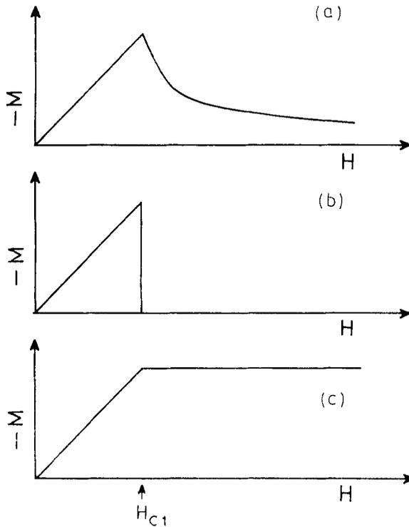
**Figure 1.** (a) Thermodynamic magnetization curve of a type-II superconductor. The detailed shape depends on the Ginzburg-Landau parameters. (b) is the approximation used by Bean (1962), while (c) is the other extreme approximation possible.
