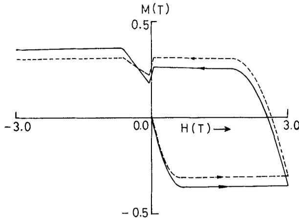
**Figure 4.** Virgin and hysteresis magnetization curves with critical current density (or  $H^*$ ) independent of magnetic field (Bean's 1964 approximation).
