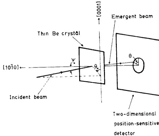
**Figure 1.** Schematic diagram of an experimental arrangement for measuring the transmission spectra of axially channelled ions in a thin Be crystal.
