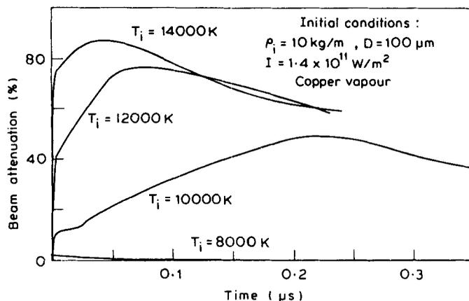
Figure 9. Beam attenuation at the surface for a range of initial temperatures.
