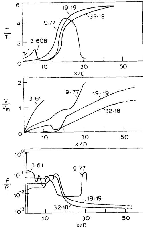
Figure 8. Plug expansion at  $t/\tau$  for  $\rho_i = 100 \text{ kg/m}^3$ ; Initial conditions;  $T_i = 10000 \text{ K}$ ;  $D = 100 \mu\text{m}$ ;  $I = 1.4 \times 10^{11} \text{ W/m}^2$ ;  $\tau = 0.059 \mu\text{s}$ ;  $V_m = 3961 \text{ m/s}$ , titanium vapour.
