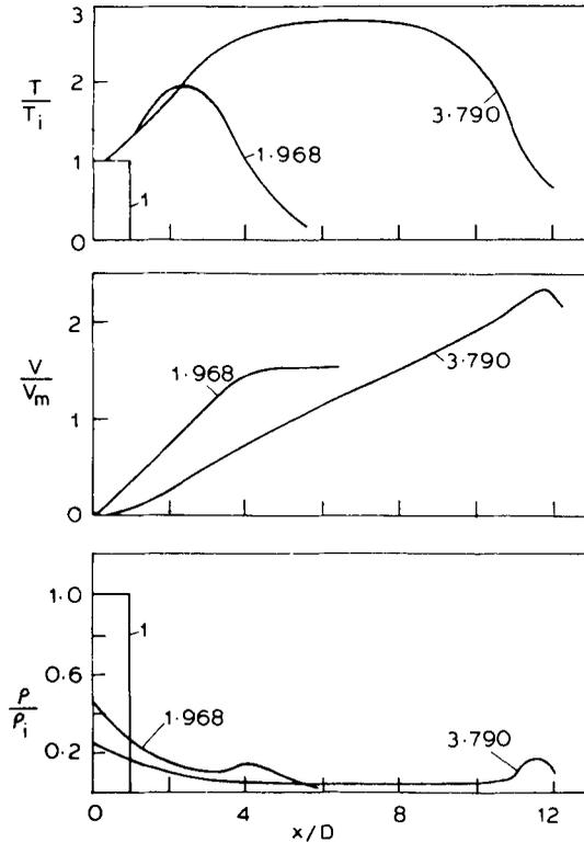
**Figure 3.** Plug expansion at  $t/\tau$  for titanium vapour. Initial conditions:  $\rho_i = 10 \text{ kg/m}^3$ ;  $T_i = 10000 \text{ K}$ ;  $D = 100 \text{ }\mu\text{m}$ ;  $I = 1.4 \times 10^{11} \text{ W/m}^2$ ;  $\tau = 0.058 \text{ }\mu\text{s}$ ;  $V_m = 3322 \text{ m/s}$ .
