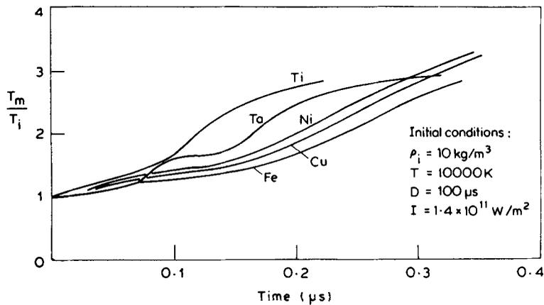
Figure 6. Variation of instantaneous maximum temperature ( $T_m$ ) for a range of metals.
