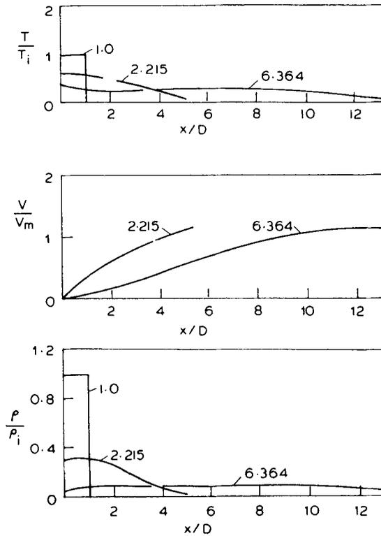
Figure 5. Plug expansion at  $t/\tau$  for copper vapour. Initial conditions:  $\rho_i = 10 \text{ kg/m}^3$ ;  $T_i = 8000 \text{ K}$ ;  $D = 100 \mu\text{m}$ ;  $I = 1.4 \times 10^{11} \text{ W/m}^2$ ;  $\tau = 0.075 \mu\text{s}$ ;  $V_m = 2400 \text{ m/s}$ , copper vapour.
