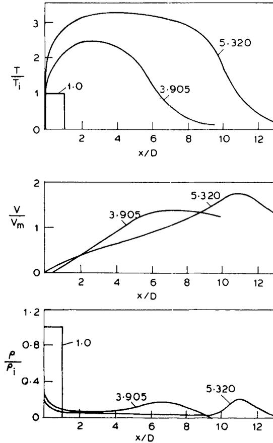
Figure 2. Plug expansion at  $t/\tau$  for  $T_i = 10000$  K;  $\rho_i = 10$  kg/m<sup>3</sup>;  $D = 100$   $\mu$ m;  $I = 1.4 \times 10^{11}$  W/m<sup>2</sup>;  $\tau = 0.068$   $\mu$ s;  $V_m = 2773$  m/s; copper vapour.
