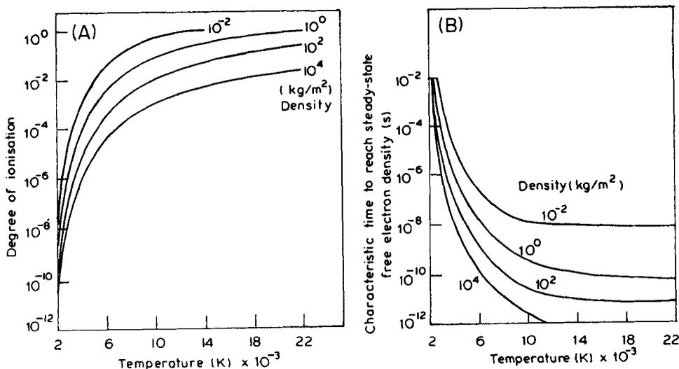
Figure 1. Degree of ionization and characteristic time for copper vapour.
