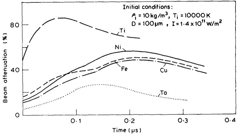
Figure 7. Beam attenuation at the surface for a range of metals.
