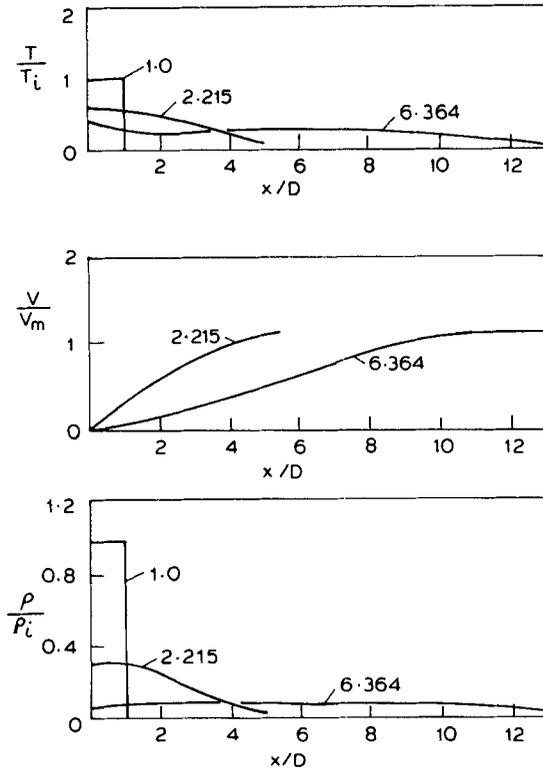
Figure 4. Plug expansion at  $t/\tau$  for  $T_i = 80000$  K. Initial conditions:  $\rho_i = 10$  kg/m<sup>3</sup>;  $D = 100$   $\mu$ m;  $I = 1.4 \times 10^{11}$  W/m<sup>2</sup>;  $\tau = 0.075$   $\mu$ s;  $V_m = 2400$  m/s, copper vapour.
