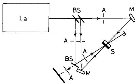
**Figure 4.** Beam geometry for OPC by degenerate four-wave mixing. M, mirror; BS, beam splitters; S, sample; A, apertures; La, laser.
