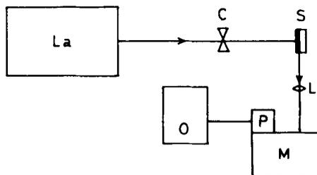
**Figure 3.** Experimental set-up for recording the oscillograms of the fluorescence emission, shown in figures 2(b) to (d). C, chopper; S, sample; L, lens; P, photomultiplier tube; M, monochromator; O, oscilloscope; La, laser.
