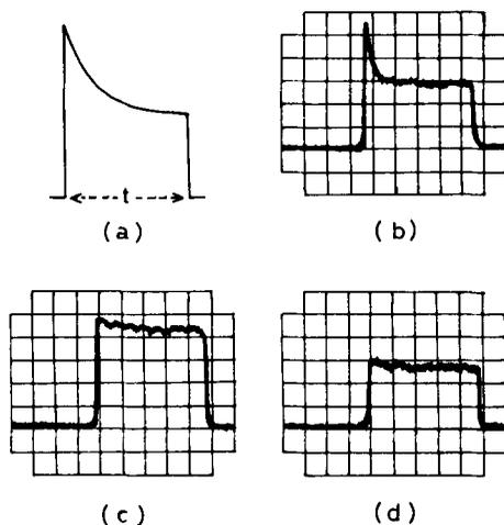
**Figure 2.** (a) Calculated fluorescence emission from a sample with  $p_1 = 10^8$ ,  $p_2 = 10^7$ ,  $p_3 = 2 \times 10^4$  and  $w = 10^4$ , for a time  $t = 5$  ms. (b) Fluorescence emission from an eosin/gelatin film, excited by 514.5 nm of argon ion laser at 500 mW power. Sweep rate: 1 ms/div. (c) Fluorescence emission from a Rhodamine 6G/gelatin film under the same conditions. (d) Fluorescence emission from an eosin/gelatin film, excited by the above laser at about 20 mW power.
