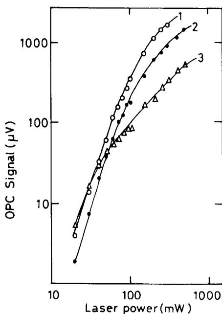
**Figure 5.** OPC signals from (1) erythrosin B, (2) Rose Bengal and (3) eosin in PVA films vs laser power.
