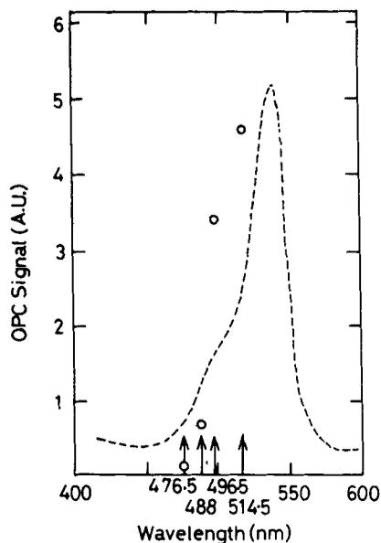
**Figure 6.** OPC signals from erythrosin B/PVA film, at the different argon ion laser wavelengths, plotted in the background of the absorption spectrum (broken line).
