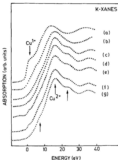
**Figure 1.** K-absorption edge region of Cu in (a)  $\text{Cu}_2\text{O}$ , (b)  $\text{CuO}$ , (c)  $\text{YBa}_2\text{Cu}_3\text{O}_{7-\delta}$  annealed in oxygen, (d)  $\text{YBa}_2\text{Cu}_3\text{O}_{7-\delta}$  annealed in air, (e)  $\text{Y}_{0.925}\text{Ce}_{0.075}\text{Ba}_2\text{Cu}_3\text{O}_{7-\delta}$ , (f)  $\text{YBa}_2\text{Cu}_3\text{O}_{7-\delta}$  quenched from  $> 870^\circ\text{C}$  and (g)  $\text{Y}_2\text{BaCuO}_5$ .
