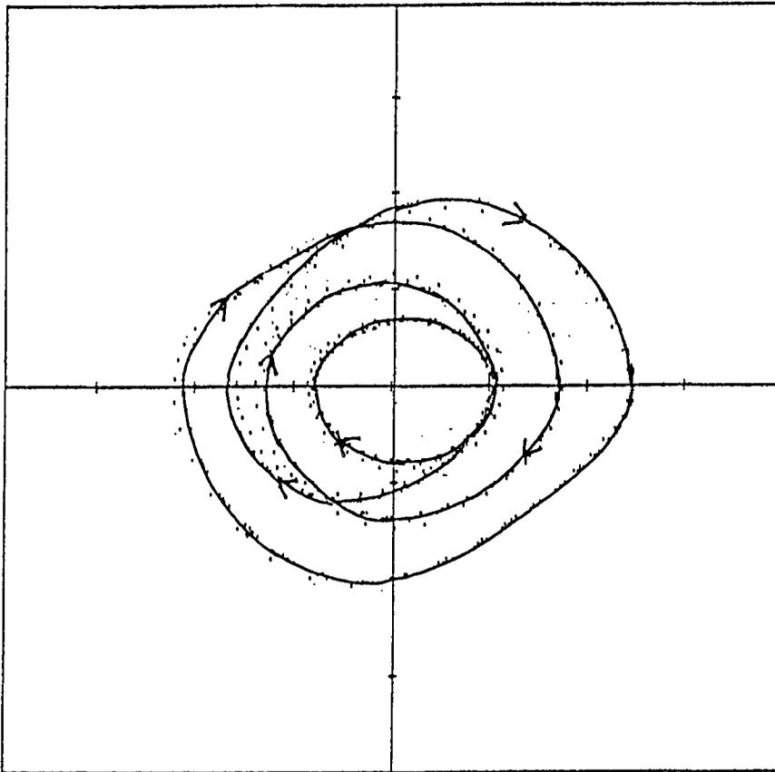
Figure 4. Asymptotic four-cycle observed at  $\beta = 0.2$ ,  $\omega = 1$  and  $A = 0.3$ .
