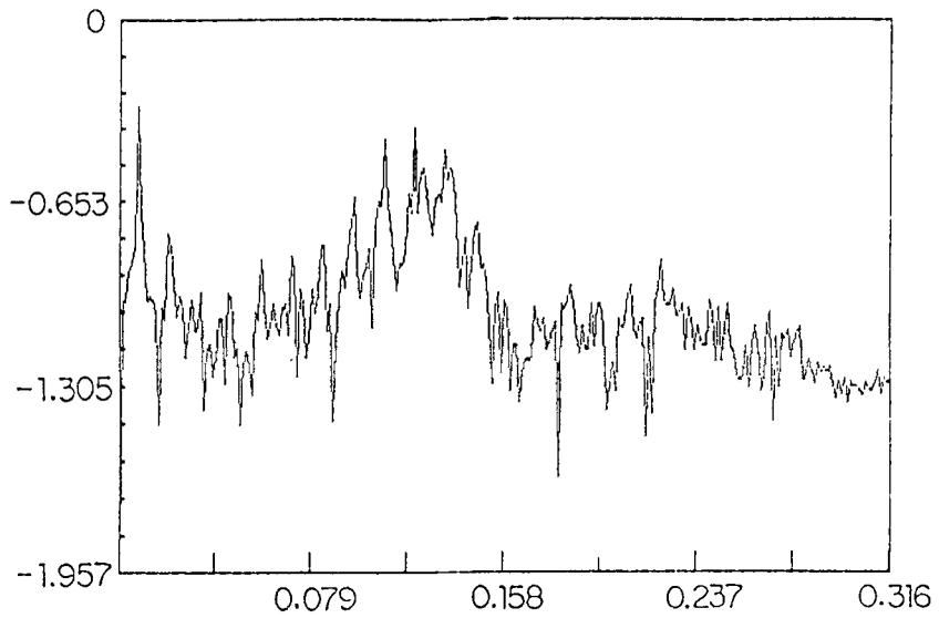
**Figure 2b.** Power spectrum using FFT of the chaotic attractor given in figure 2a. Log(power) is plotted along the y-axis with frequency along the x-axis.
