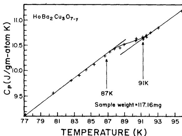
**Figure 2.** Heat capacity  $C_p$  of the sample of  $\text{HoBa}_2\text{Cu}_3\text{O}_{7-y}$ . The line drawn through the experimental points is a guide to the eye.
