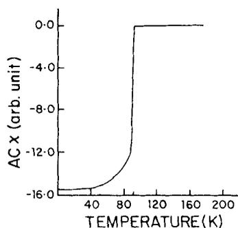
**Figure 1.** AC susceptibility of a single phase sample of  $\text{HoBa}_2\text{Cu}_3\text{O}_{7-y}$ . The strong diamagnetic response of the sample (in the neighbourhood of  $T = 91$  K) gives the superconducting transition temperature  $T_c = 91$  K.
