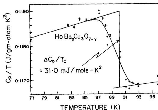
**Figure 3.**  $C_p/T$  of  $\text{HoBa}_2\text{Cu}_3\text{O}_{7-y}$ . The jump in heat capacity  $\Delta C_p/T_c$  can be seen very conveniently.
