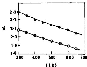
Figure 3. Grüneisen parameters of  $\text{CdF}_2$  (closed circle) and  $\text{PbF}_2$  (open circle) as a function of temperature.
