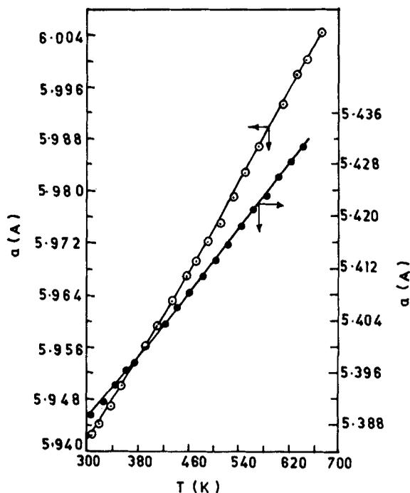
**Figure 1.** Lattice parameters of  $\text{CdF}_2$  (closed circle) and  $\text{PbF}_2$  (open circle) at various temperatures.
