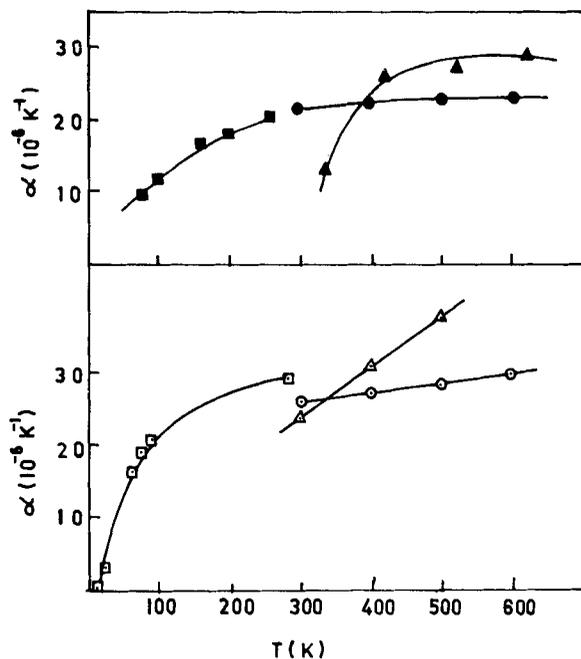
**Figure 2.** Temperature variation of coefficient of thermal expansion of  $\text{CdF}_2$  and  $\text{PbF}_2$  ( $\text{CdF}_2$ : closed circle, present work; closed square, Shaharbany (1976); closed triangle, Krukowska-Fulde and Niemyski (1967).  $\text{PbF}_2$ : open circle, present work; open square, White (1980); open triangle, Aurora (1984).
