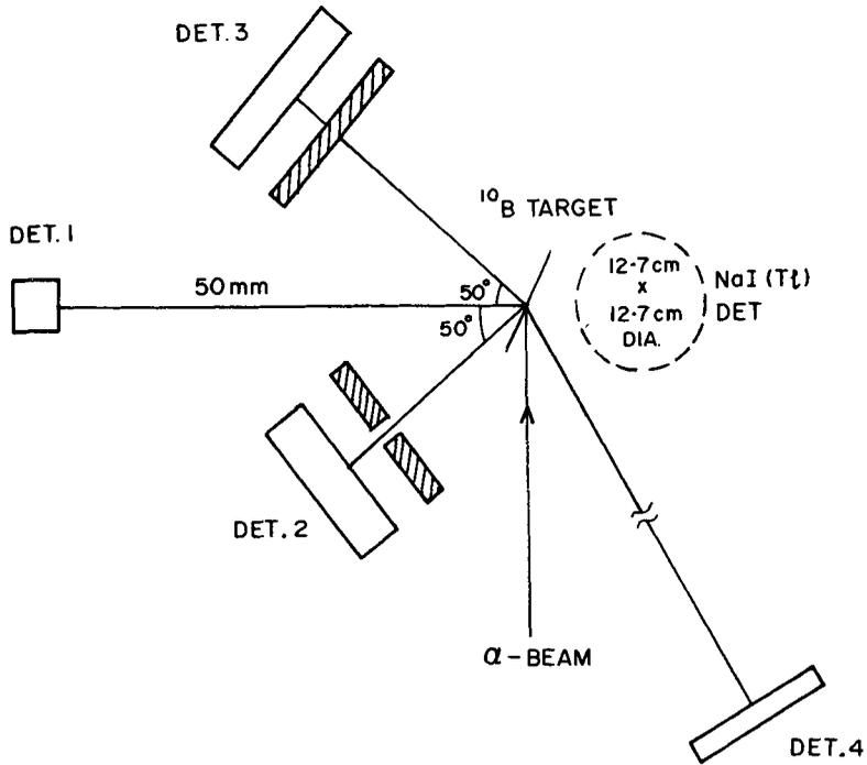
**Figure 1.** Schematic diagram of the experimental configuration. Detectors 1, 2 and 3 are liquid nitrogen cooled Si(Li) detectors. Detector 4 is a Si surface barrier detector. In addition to the NaI(Tl) detector, a 120 cm<sup>3</sup> Ge(Li) detector was also used for detecting gamma rays.
