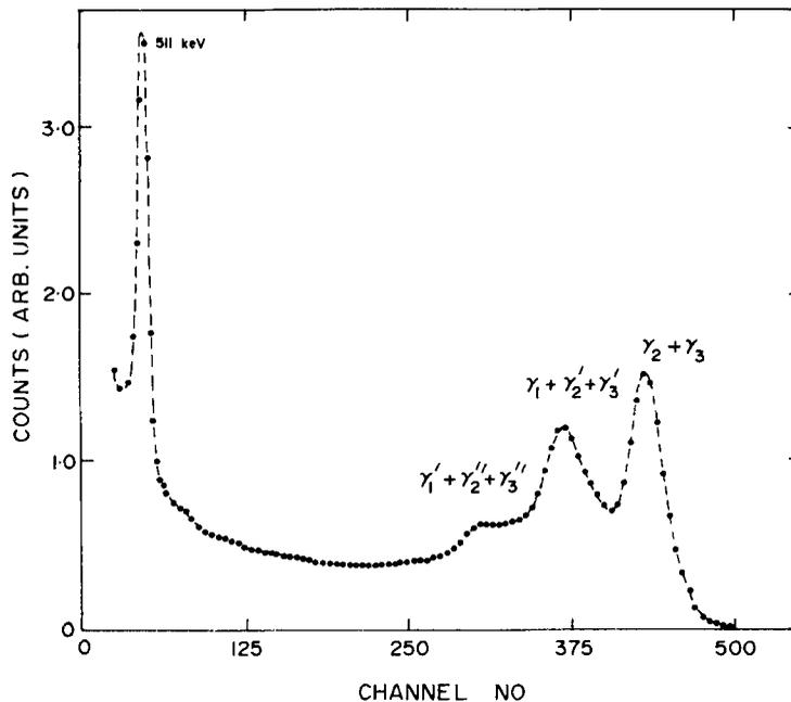
Figure 3. Gamma spectrum obtained with a NaI(Tl) detector at  $E_\alpha = 2.31$  MeV.
