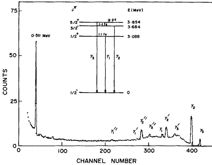
Figure 4. Gamma spectrum obtained with a Ge(Li) detector at  $E_x = 2.31$  MeV. The observed peaks all correspond to the reaction under study.
